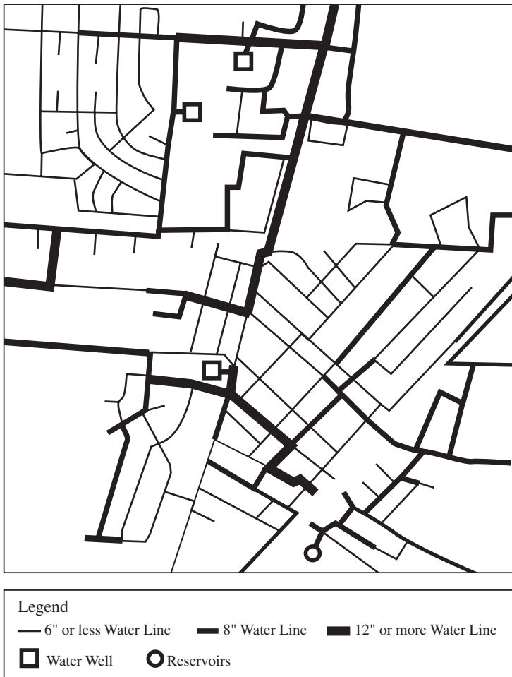
Fig. 7–3. Example of a water system map
