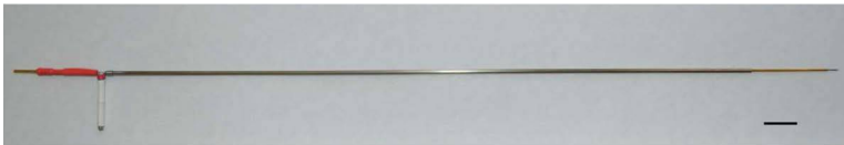
Figure 20.3 Electrophysiology targeting electrode. The exposed tungsten tip is at right (though too small to see at this resolution), the electrical contacts at left. The red contact at left is connected to the tungsten tip, while the white contact at left-bottom is connected to a stainless steel jacket coaxial with the tungsten tip. In use, this electrode is inserted into the brain through a stainless steel cannula, which is held in place by a stereotactic surgical frame. The black scale bar at the lower-right is 1 cm.
