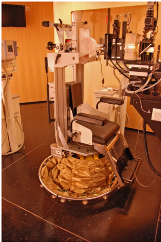
Figure 9.5 The treatment chair and nozzle for the OPTIS facility at PSI. This is a passive scattering facility dedicated to the treatment of uveal melanomas, which are rather aggressive tumors of the retina.
