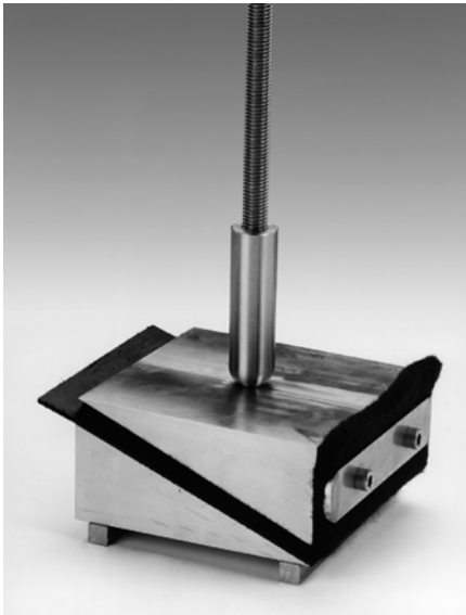
Fig. 3.23. Details of the specimen holder. The top wedge is kept in position just by the friction force between geomembrane on the bottom wedge and nonwoven geotextile fixed on the bottom surface of the top wedge
