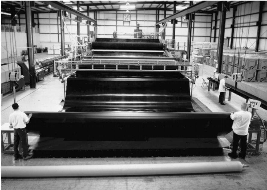
Fig. 2.10. Cooling system line of a production unit for 7 m wide geomembranes. Behind the cooling and polishing roll stack the geomembrane first passes through an ambient temperature cooling line, which can be as long as 20 m depending upon the size of the equipment, and continues to be cooled down by the ambient air. At the end of the cooling line the geomembrane is rolled up on a take-up spool (foreground). Typically 100 to 150 m long geomembranes are manufactured. Roll changes take place every 1 to 2 hours. In each case a cross-stripe is cut off to be tested in the manufacture quality assurance laboratory. The roll is often wrapped. If the properties are satisfactory according to various test results, the roll is released and transported to the delivery store
