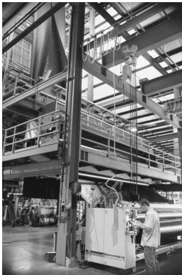
Fig. 2.11. View of a blown sheet extrusion line. In the background, bottom left, the circular die can be seen of which an HDPE hose, supported by supporting air, exits. The cut tube runs down from the top and covers the view onto the closed tube running upward into the layflat boards. The cut hose enters the take-up mechanism (middle ground) and is finally wound on a spool in the winding mechanism (foreground). The plant tower may be as high as 40 m and is visible on the factory site from a great distance. Figs 2.10 and 2.11 courtesy Serrot International
