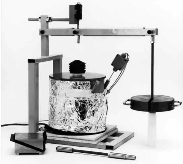
Fig. 3.22. Test device for long-term shear test with all components
