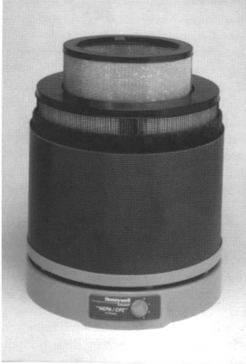
Figure 6-1 Room-size high-efficiency particulate air (HEPA) filtering system. This self-contained system features a circulating fan and a HEPA filter, plus a charcoal prefilter. The use of such a room-size system may allow patients to turn their bedrooms into "safe havens" when they are unable to install central HEPA filtration systems. (Courtesy of Allergy Control Products Inc., 96 Danbury Road, Ridgefield, CT 06877.)
