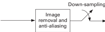
Figure 12.6 Block diagram of the sample rate conversion module in DDC when the conversion rate is an integer.
