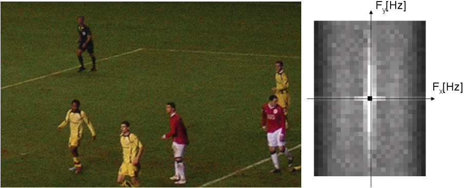
Fig. 1. noisy PAL broadcast of a sports event and PSD of noise in a green color channel of the PAL broadcast.
