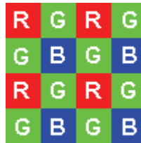
Fig. 2. Bayer mosaic pattern of photosensitive elements in a camera sensor
