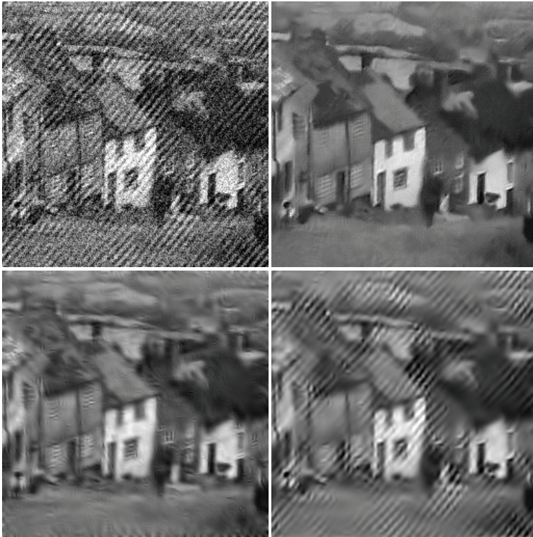
Fig. 16. Denoising results of Goldhill image corrupted by heavily correlated streak noise (top left): by NLMS denoising (top right), by BLS-GSM denoising (bottom left), by Probshrink denoising for white noise (bottom right)
