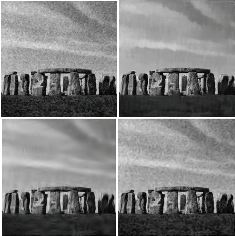
Fig. 17. Denoising results of Stonehenge image corrupted by simulated red channel demosaicing noise (top left): by NLMS denoising (top right), by BLS-GSM denoising (bottom left), by Probshrink denoising for white noise (bottom right)
