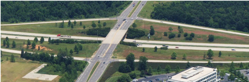
Figure 4.47 Interchange with underpass (major road under).
