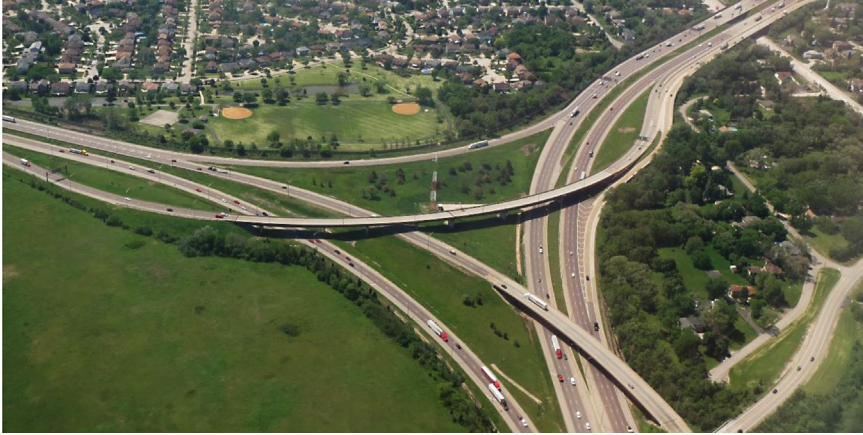
Figure 4.41 Directional three-leg interchange.
