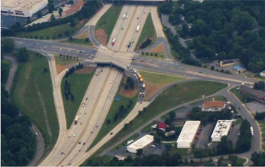
Figure 4.45 Single point interchange.
