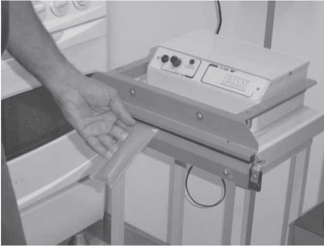
FIG. 25.1. Detail showing heat-sealing of polyethylene bags with passion fruit purée
