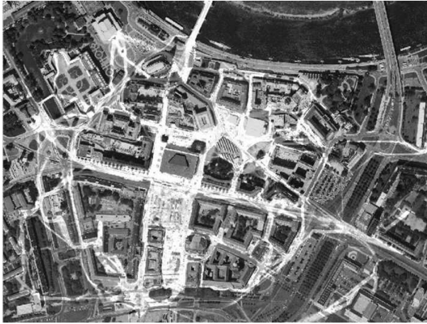
Fig. 6. Densities of pedestrian streams in a simulation of the city center of Dresden, Germany. Our simulation includes 30.000 pedestrians (after Helbing et al. 2005d).
