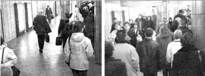
Fig. 7. The interfaces of opposite pedestrian flows can be efficiently stabilized by a series of columns (here in a tunnel of the metro system of Budapest at Deak Tér). Nevertheless, the permeability allows for a flexible usage in accordance with the respective pedestrian traffic volumes in both directions (after Helbing et al. 2005a).
