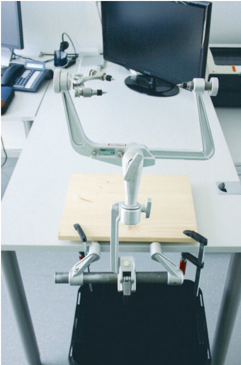
Fig. 2.1 Fixation of the Mayfield clamp to an office desk with screw clamps.
