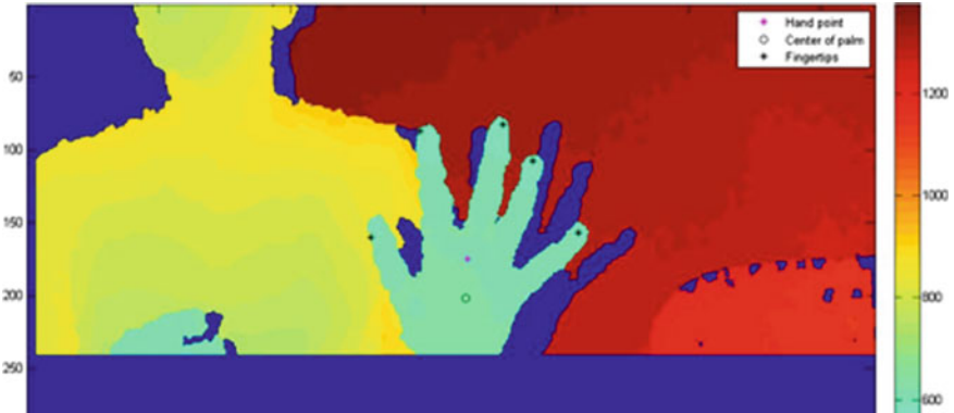
Fig. 6.10 Final result showing hand point, the center of palm, and fingertips
