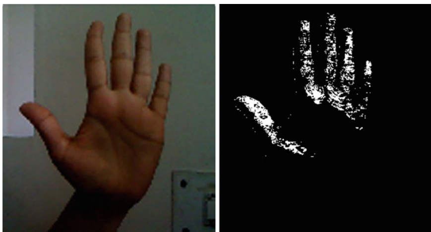
Fig. 5.14 Test image captured at real time and output after skin filtering
