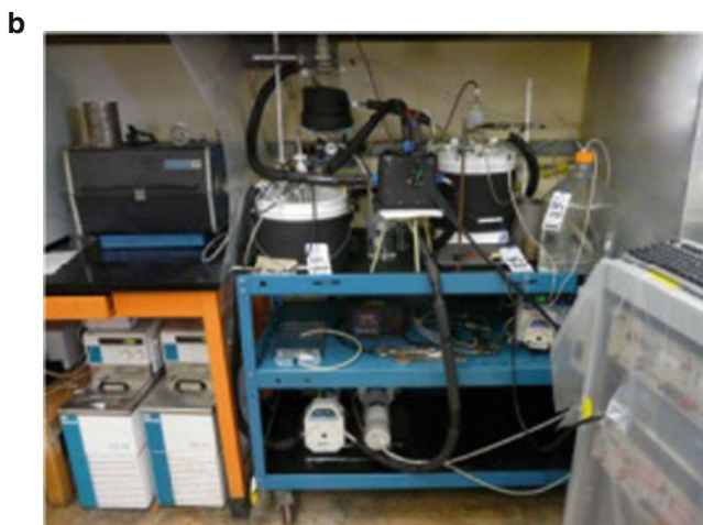
Fig. 6.26 Experimental facility at AECL for testing a single-cell electrolyzer for the CuCl/HCl solution: (a) system diagram (modified from Naterer et al. 2011a), (b) photograph (courtesy of S. Suppiah)
