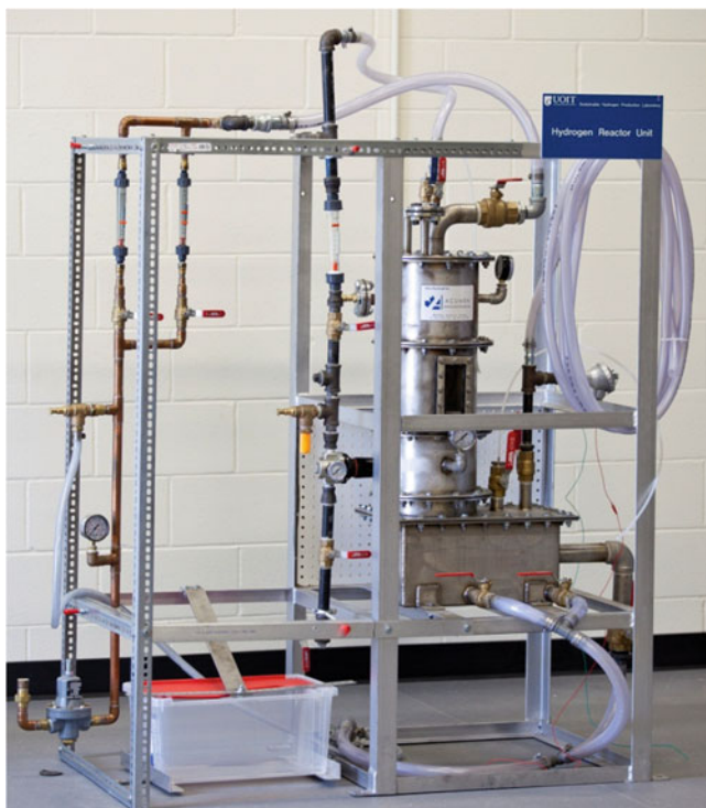
Fig. 6.80 Scaled-up reactor for thermochemical chlorination step (UOIT)
