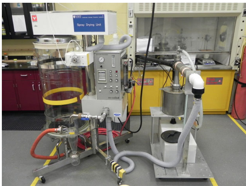
Fig. 6.69 Photograph of the experimental spray drying unit for \text{CuCl}_2 \cdot n\text{H}_2\text{O} dehydration at UOIT
