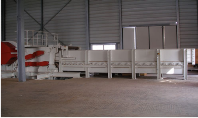
Fig. 6.8 Drum chipper with feed belt by Rudnick & Emmers [2]
