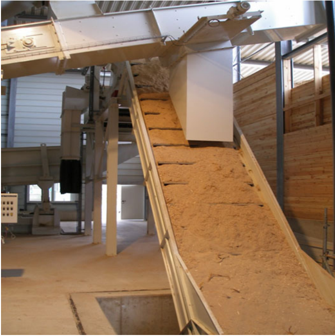
Fig. 6.21 Scraper chain conveyor with chips, by Rudnick & Enners
