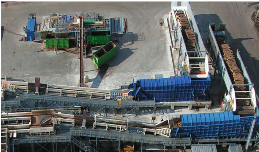
Fig. 6.7 Debarking using a rotary debarker in two lines [1]
