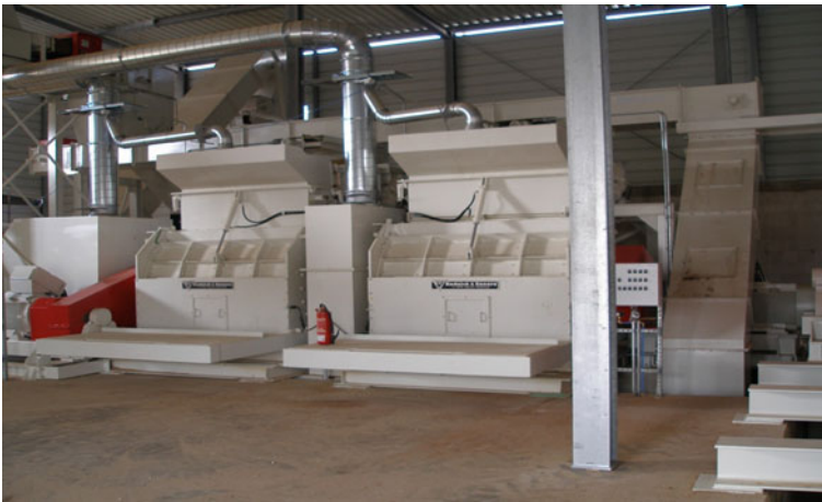
Fig. 6.13 Wet hammer mills by Rudnick & Enners [2]
