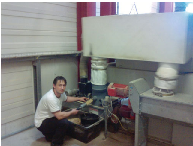
Fig. 6.42 Sampling directly below the pellet sieve
