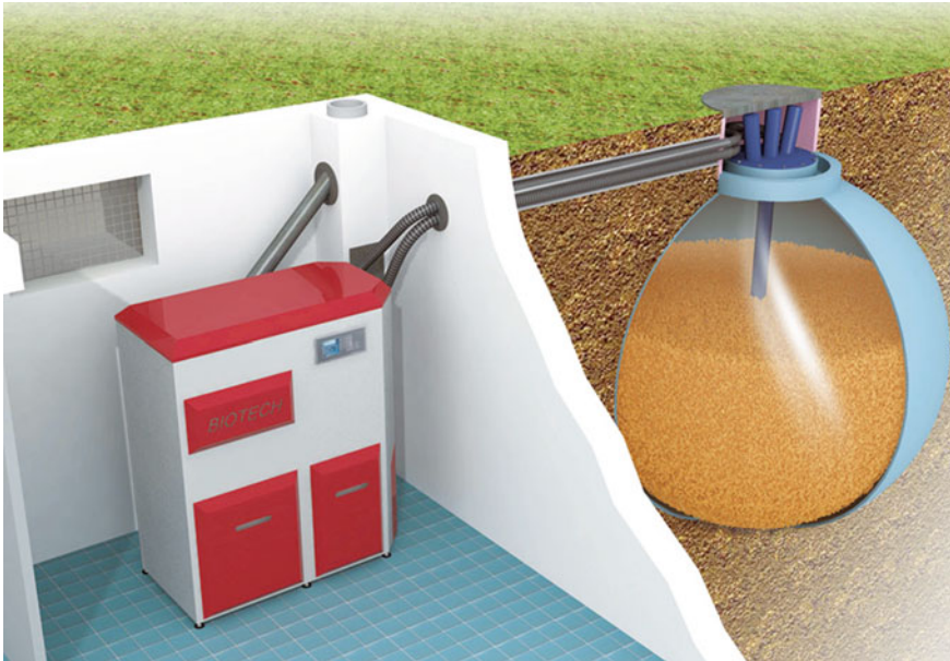
Fig. 7.8 Buried tank for external pellet storage [2]
