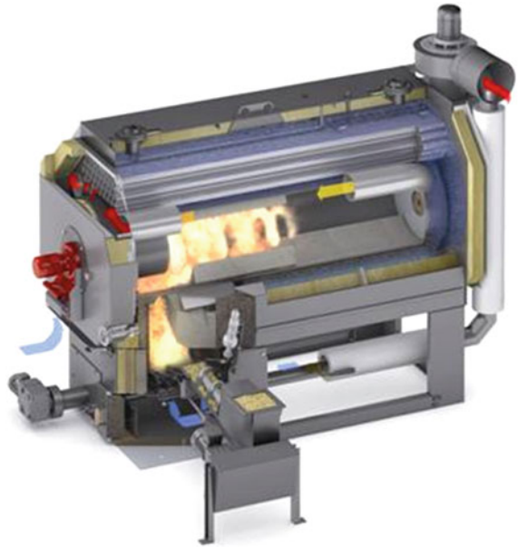
Fig. 7.24 Pellet firing system according to the rotary firing system principle. Type Pyrot by KÖB/ Viessmann [11]
