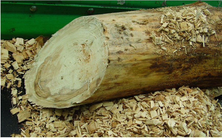
Fig. 6.10 Log wood and wood chips after use of a chipper
