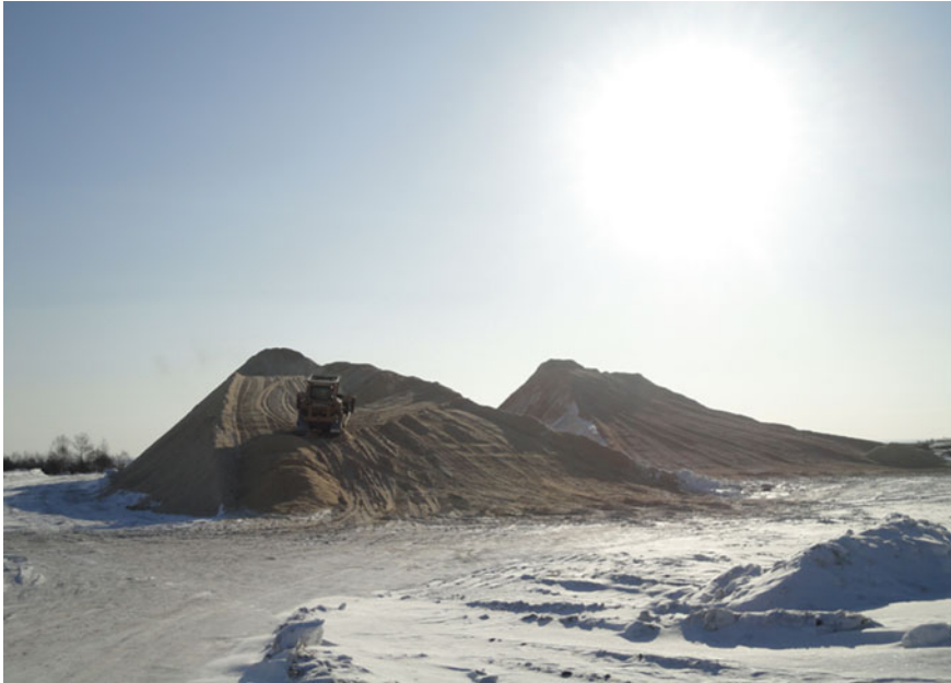
Fig. 6.14 Open-air storage on sealed ground without boundary walls
