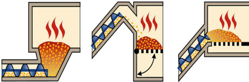
Fig. 7.11 Principle of the various pellet burners (Solarpraxis) [4]: Left —Underfeed burner, Centre —Drop shaft burner, Right —Retort burner with pellet side entry
