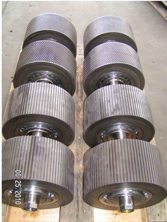
Fig. 6.55 Top: Perforated edge runner; Bottom: straight-fluted edge runner, by Salmatec [6]
