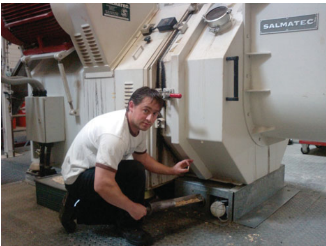
Fig. 6.41 Sampling directly below the presses
