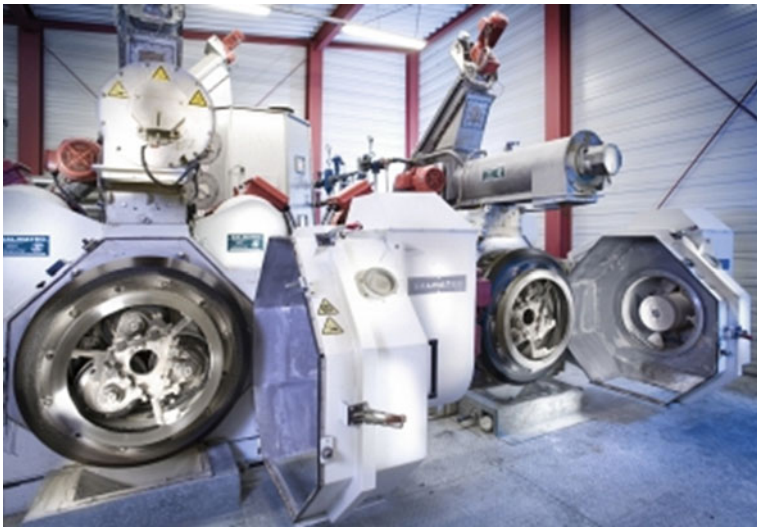
Fig. 6.59 Two presses with three edge runners each
