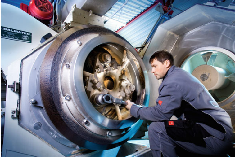
Fig. 6.58 Adjusting the edge runner position
