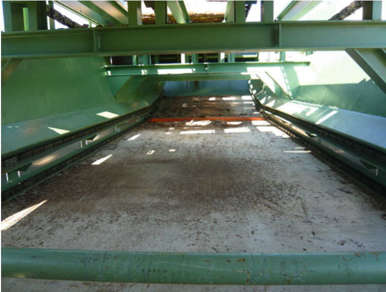
Fig. 6.19 Scraper-floor construction by Holtec [1]
