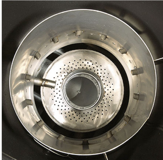
Fig. 7.13 Arrangement of the secondary-air nozzles in the post-combustion ring by KWB [5]
