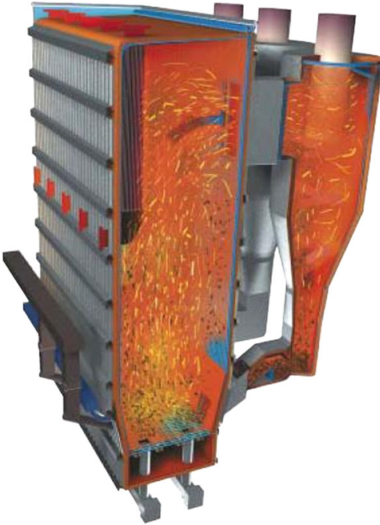
Fig. 7.34 Circulating fluidized-bed firing system by Metso Power [16]
