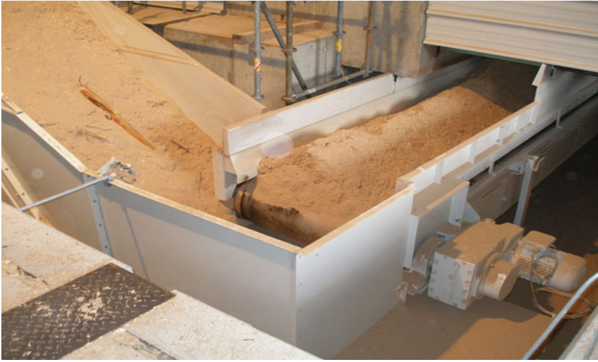
Fig. 6.22 Conveyor belt for high chip capacities behind a push floor, by Rudnick & Enners
