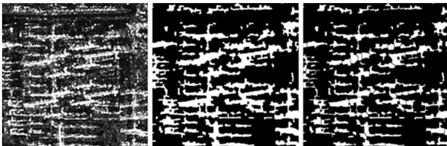
Fig. 65.2 Left TerraSAR-X intensity SAR image of a part of the test site. Middle Building detection result of the left image. Right Result of splitting big-size light region with our hybrid morphological operators
