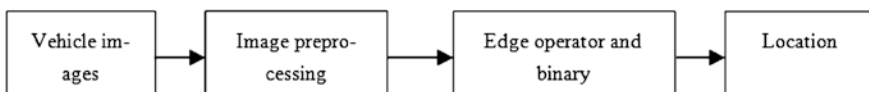
Fig. 48.1 The process of the algorithm of license plate location based on edge detection
