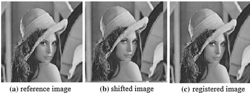
Fig. 64.1 Reference images (a), the object image (b), and after shifted (5.65, 12.09) and the registered image (c) with \lambda = 100
