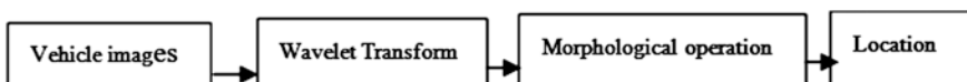
Fig. 48.3 The process of the algorithm of license plate location based on wavelet transform
