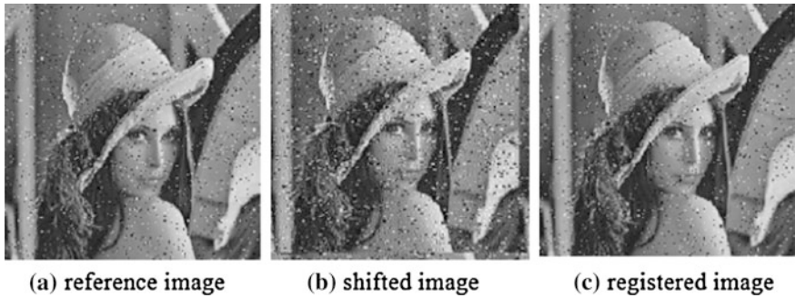
Fig. 64.3 Reference images (a) with salt noise, the object image (b), and after shifted (9.49543, 8.7465) and the registered image (c) with \lambda = 100
