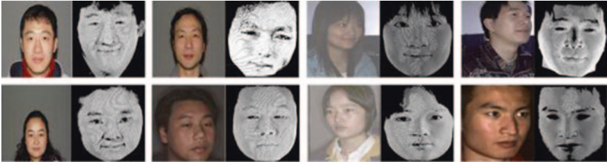
Fig. 59.1 SFS-based depth recovery results: the left image is the input 2D gray image and the right image is the facial surface depth recovered by SFS
