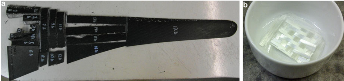
Fig. 5.1 (a) Cut blade with part labels. Parts c1 and c2 were used for compression testing of the core, 7,9 and 11 for tensile testing of the core and 13b, 13f, 14b, 14f and 15f for tensile testing of the skin, where f and b denotes front and back surface, respectively. (b) Glass fibre content of blade
