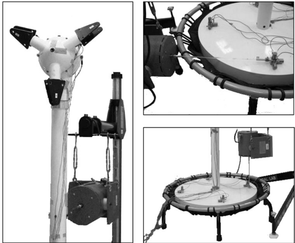
Fig. 16.4 Drive points to excite rigid body modes: tower for pitching and rolling modes ( left ) and base for yawing ( top right ) and y-direction bounce ( bottom right )
