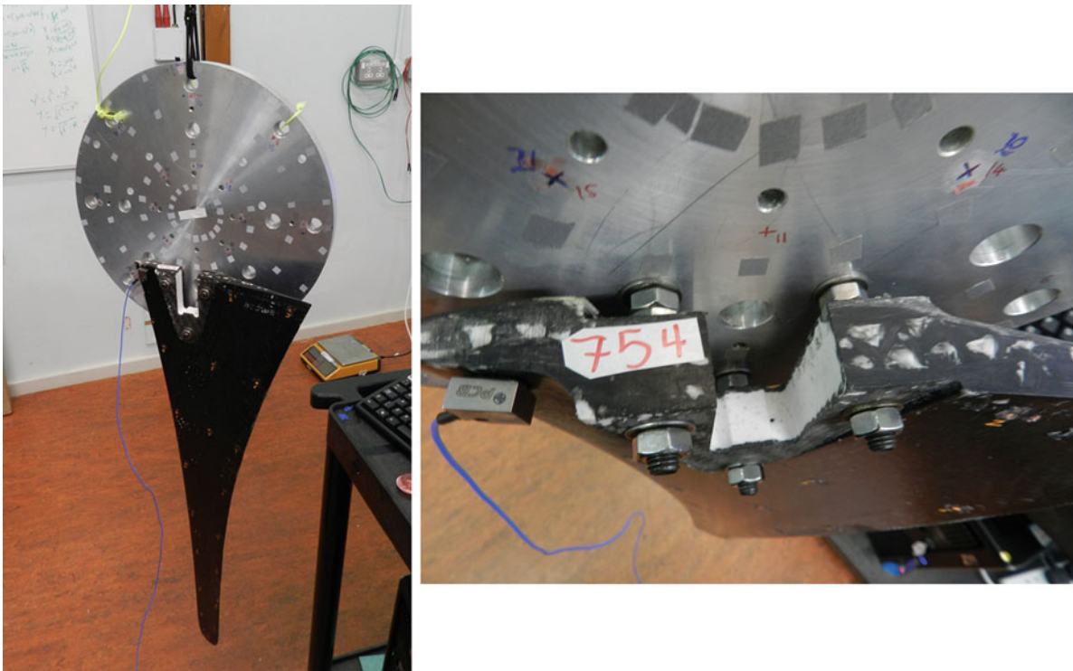
Fig. 12.5 Photographs of the experimental setup for the turbine blade bolted to transmission simulator
