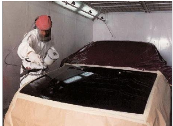
133 Paint sprayer: Isocyanates, present in the hardener or catalyst of polyurethane-based two-part paints, are one of the commonest offending agents in occupational asthma.
