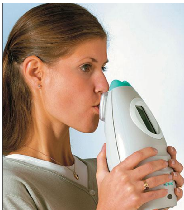
53 Exhaled nitric oxide analyser. Hand-held precalibrated monitor (Niox Mino) which delivers an accurate exhaled NO measurement within minutes. Patient inhales deeply through the disposable filter and then exhales at around 50 ml/sec. Suitable for use with adults or children.
