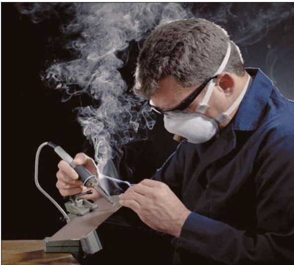
135 Colophony exposure. Colophony (also called rosin) is a natural product which comes from pine sap and is an ingredient in solder flux. It is a well-known irritant and sensitizer, and a major cause of occupational asthma. Cases of asthma due to fumes from fluxes containing aluminium have also been reported.
