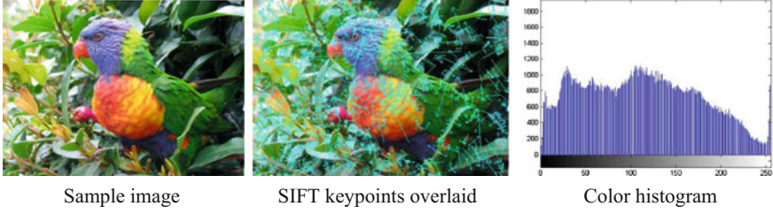
Fig. 10 A sample image from PASCAL VOC 2011 challenge [46] with its SIFT points and histogram
