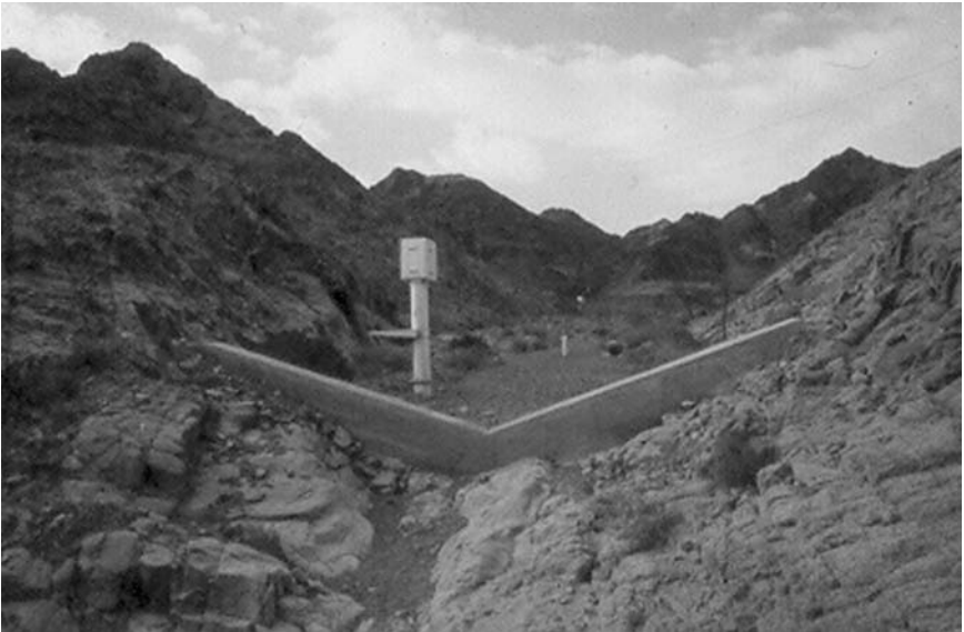
Plate 3.2 Hydrological challenges: (a) the flux away from a commercial forest as intercepted water 'steams' away; (b) waiting for flow: a measurement weir in a wadi in semi-arid Israel.
