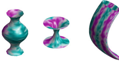
Fig. 6 On each test surface, at each of the data location \mathbf{x}_i , coinciding with the nodes of the three-dimensional meshes approximating the surface domains, independent normally distributed errors with mean zero and a standard deviation 0.5 are added to the test function; the color maps are obtained by linear interpolation of the resulting noisy observations
