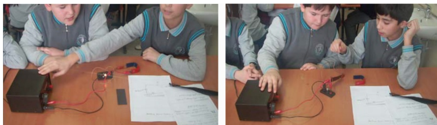
Figure 5.2. Experimental setting for testing electrical conductivity of plastic and metal magnets
