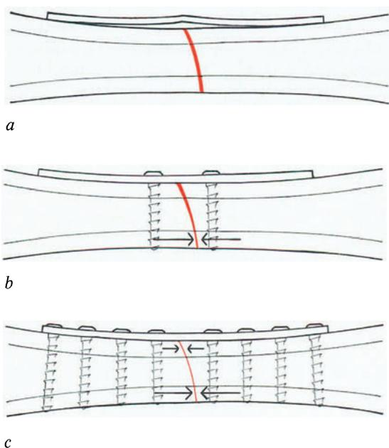
Fig. 2.16 a-c. *a* The pre-bent plate is placed over the fracture with 2 mm of overbending. *b* Insertion of the initial screws causes the plate to straighten elastically, providing compression at the *trans* cortex. *c* Placement of all the other screws adds to the straightening of the plate and provides a more uniform compression across the fracture site.
