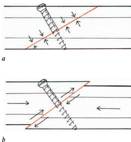
Fig. 2.11 a, b. *a* Frictional forces perpendicular to the fracture line (normal forces) will provide good stability with interfragmentary compression. *b* Superimposition of longitudinal forces may convert normal forces to shearing forces (forces parallel to the fracture line), resulting in movement at the fracture line.
