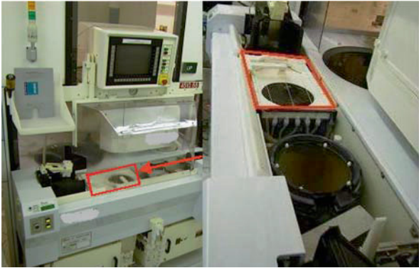
Fig. 32.3 Wet NovaScan 210 integrated on to a Westech 372
