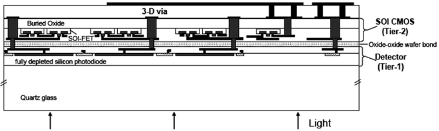
Fig. 6.10 Schematic of 3D stacked imager circuit with a Si photodetector wafer (Tier-1) and an inverted FDSOI CMOS wafer (Tier-2) [26]
