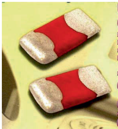
Fig. 5.5 Green anode blanks formed for pilot plant production of EPD solid electrolyte capacitors. Note the freedom from process defects
