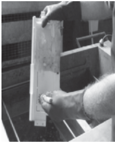
Fig. 4. The Hand clean stage to remove toner dust
