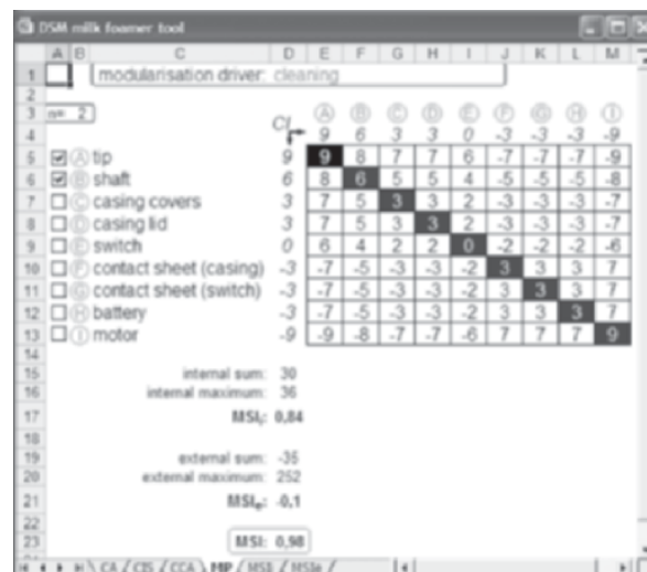
Fig. 14. Spreadsheet based calculation of modularisation configurations for the milk foamer
