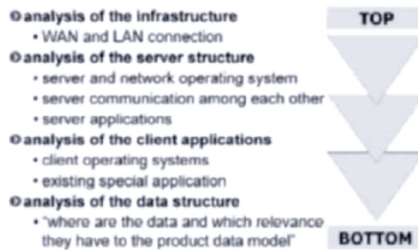
Fig. 3. Top-Down procedure for IT analysis
