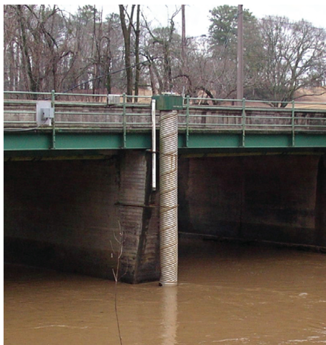
FIGURE 3.9 Typical USGS stream gage. The box on top of the metal pipe contains a data logger that has a pulley with a metal wire holding a float at one end. As the water in the stream moves up and down, the float moves, turning the pulley and changing the gage-height reading. The data are transmitted to computers via satellite radio. SOURCE: USGS.
