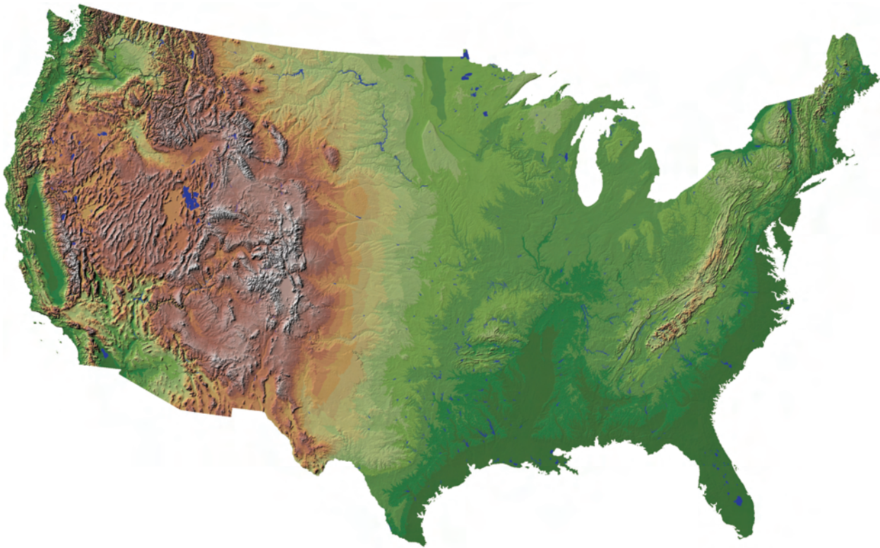
FIGURE 3.6 A shaded relief representation of the conterminous United States created from the National Elevation Dataset. Elevation is shown as a range of colors, from dark green for low elevations to white for high elevations. SOURCE: USGS, < http://erg.usgs.gov/isb/pubs/factsheets/fs10602.html >.
