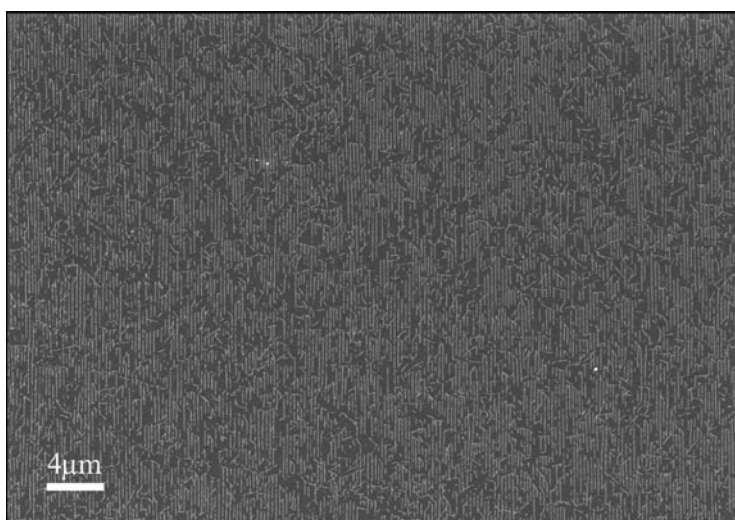
Fig. 18 Scanning electron microscopy image indicating that long-range order is preserved in the stamping process and those mesoscale dimensions can be approached using stamping
