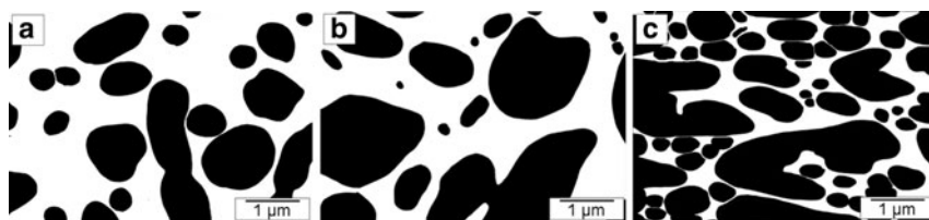
Fig. 6 Morphology of PPE/SAN blends following melt-extrusion: (a) PPE/SAN 40/60, (b) PPE/SAN 50/50, (c) PPE/SAN 60/40 (binary images of SEM micrographs: PPE – dark, SAN – bright)
