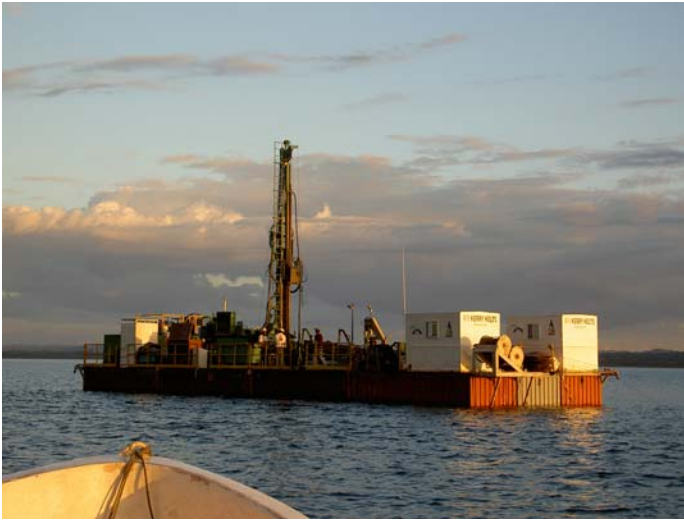
Fig. 6. The Global Lake Drilling Facility GLAD800 on Lake Peten Itza in March 2006. The system consists of a barge of shipping containers and a small wireline drilling rig (photo by J. Kueck).
