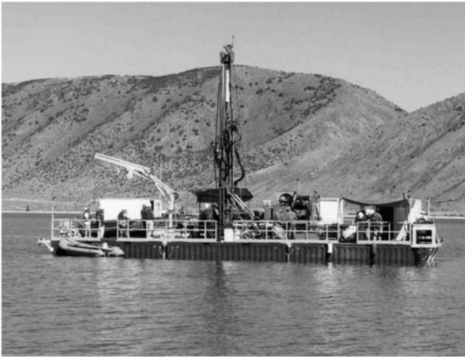
Fig. 3. GLAD800 rig and R/V Kerry Kelts during sea trial drilling at Bear Lake (photo by R. Conze).
