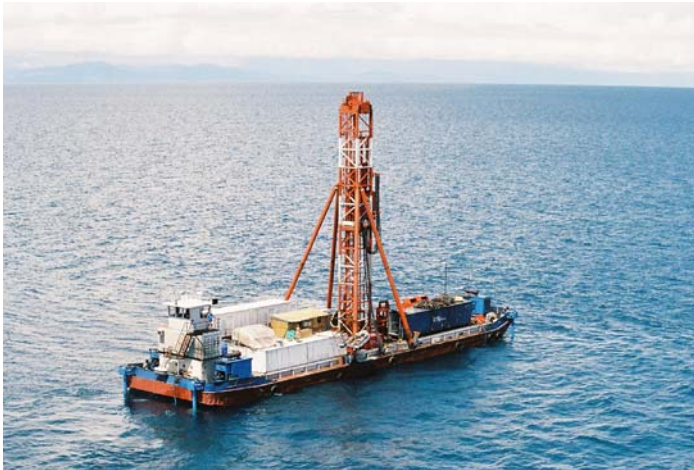
Fig. 7. Lake Malawi drilling project barge Viphya and SEACORE CS-100 drill rig on station in northern Lake Malawi with rift valley escarpment in the background. Three of the four thrust-master dynamic positioning engines (blue) are visible at the bow and stern of the barge (photo by J. Agnitch).
