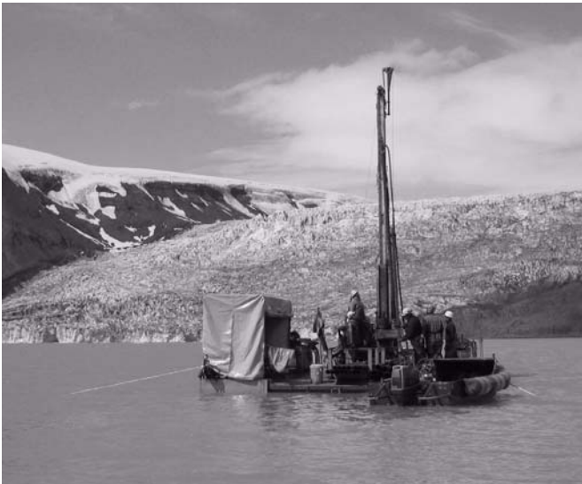
Fig. 12. The GLAD200 drilling facility on an Icelandic lake. The drill rig has a capacity of 200 m drill length, the barge is 10 by 5 m (photo by D. Nielson).
