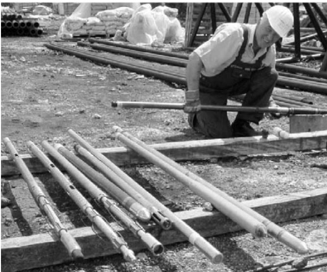
Fig. 4. Photo of slimhole geophysical logging sondes comprising electrical resistivity, natural gamma spectrum, sonic, magnetic susceptibility, magnetic field, as well as structural ultrasonic image tool.
