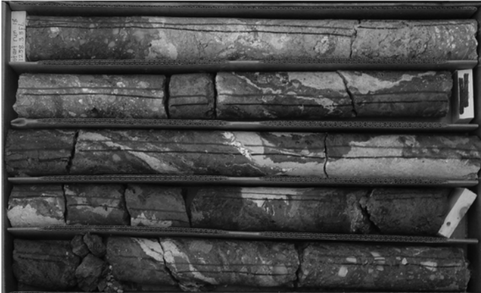
Fig. 12. Core box number 16 from corehole LB07A at Lake Bosumtwi, starting (upper left) at 383.5 m below lake surface, showing crater-fill breccia, a polymict impact breccia with some recrystallized melt (photo by C. Koeberl).
