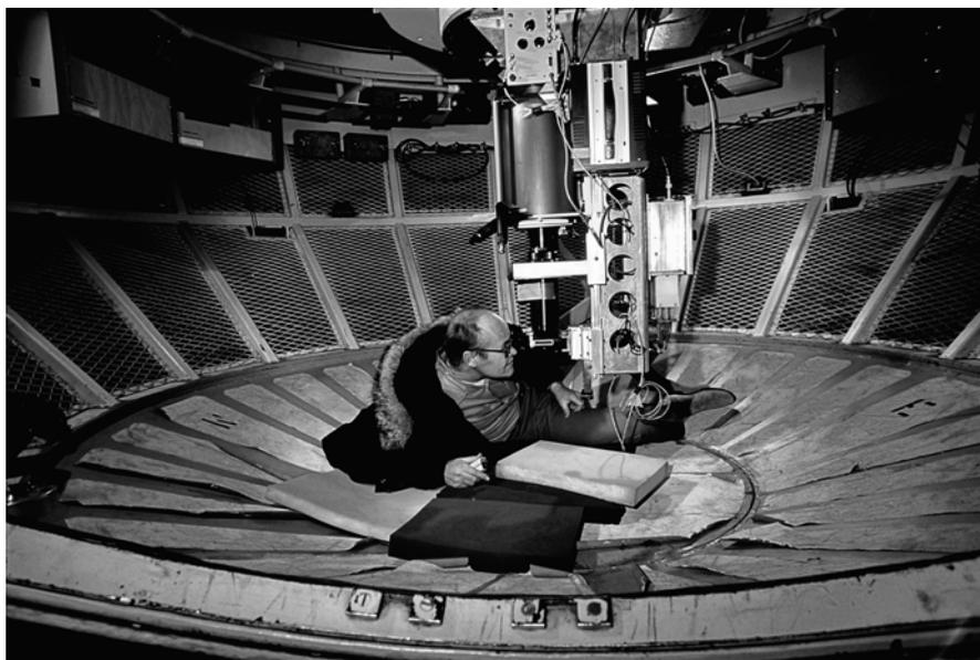
**Fig. 5.10.** Roger Lynds adjusts experimental instrumentation in the Cassegrain instrument cage of the 4-meter Mayall telescope of Kitt Peak National Observatory. Hoag's initial photographs revealing lensed arcs in clusters were taken with this telescope, which was later used by Lynds and collaborator Vahe Petrosian to measure the redshifts of arcs and confirm their lensed nature. (NOAO/AURA/NSF, used by permission of NOAO and R. Lynds.)
