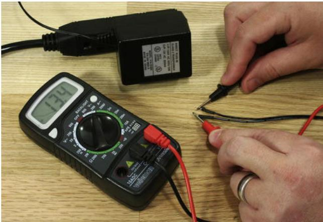
**Figure 7-11.** *Measuring AC adapter voltage*
