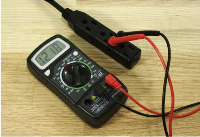
**Figure 7-10.** *Measuring AC mains voltage*
