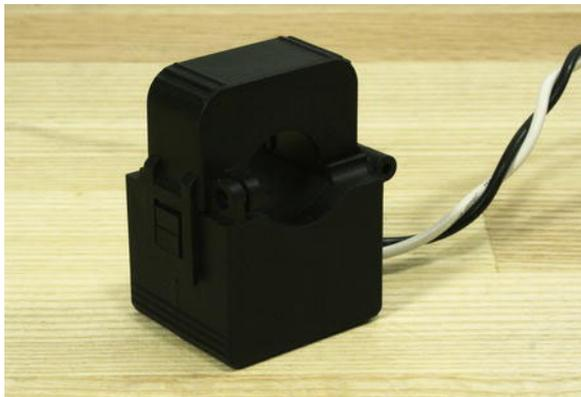
**Figure 7-1.** A 100 amp, 333 millivolt output, split-core current transformer
