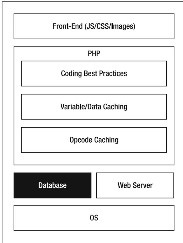
*Figure 8–1. PHP application component stack*
