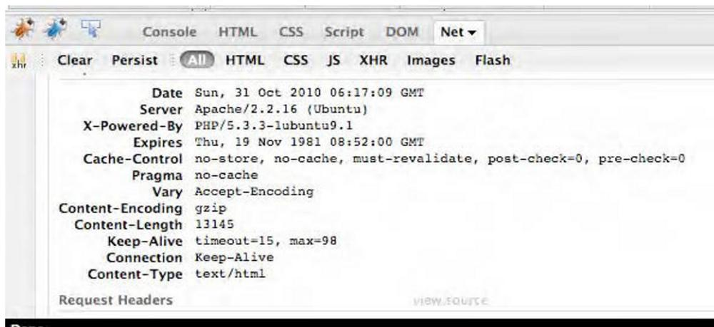
Figure 7-1. Firebug showing a Content-Encoding value of gzip
