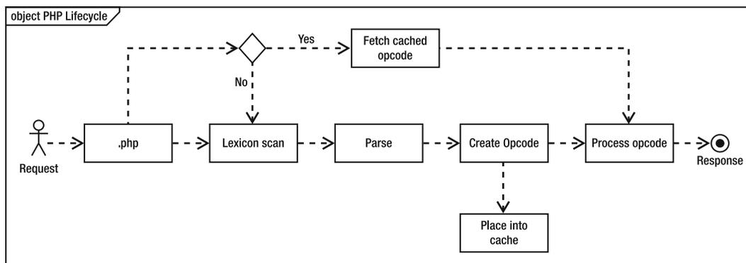
**Figure 4–3.** PHP life cycle with Opcode caching
