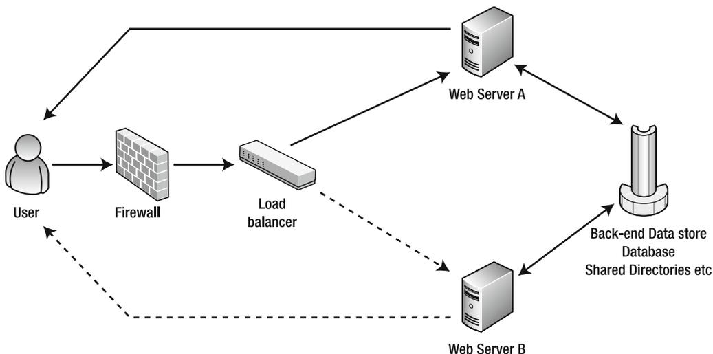
**Figure 7-3.** Distributed web application with direct server return
