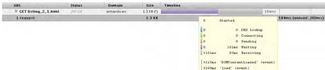
Figure 2–13. Firebug net results for Listing 2–1
