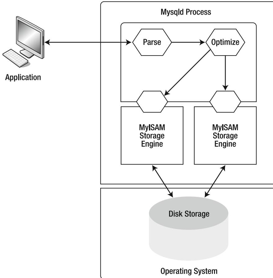
*Figure 8–2. mysqld process and storage engines*
