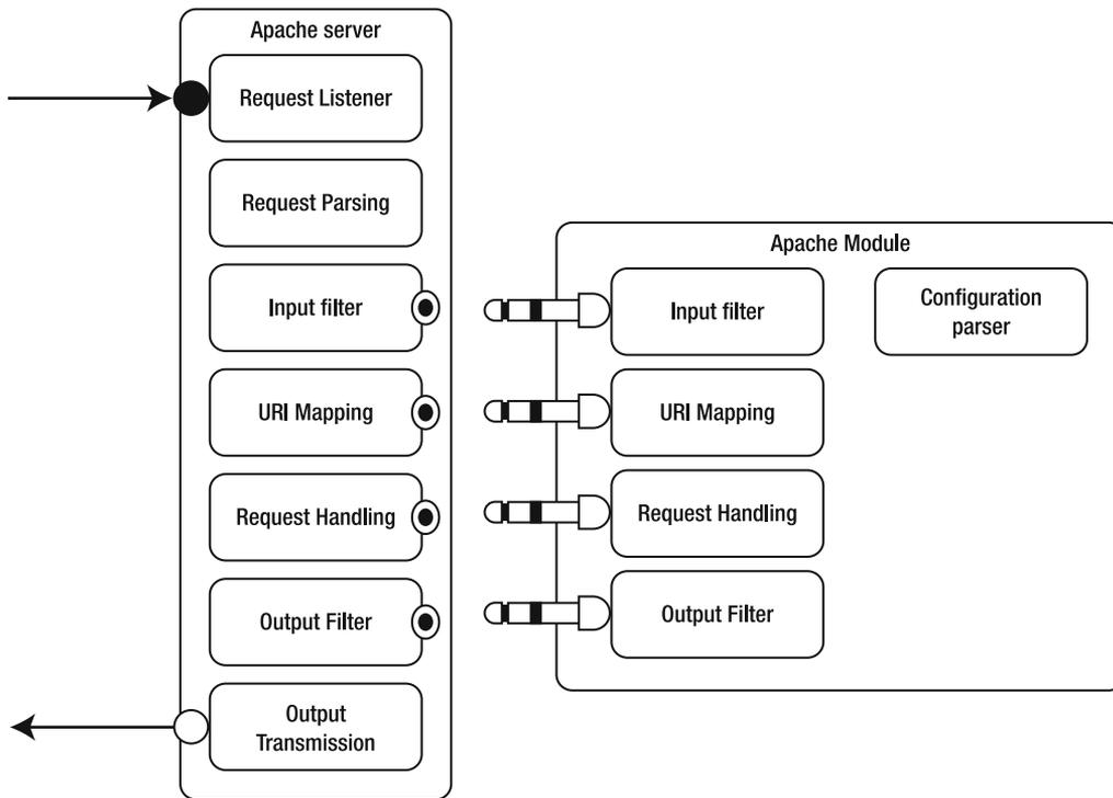
*Figure 6–3. Apache module attachment to processing pipeline*
