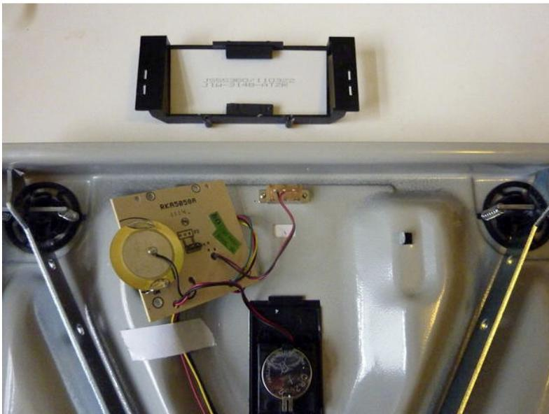
*Figure 10-2. Scale after removing the cover and LCD*
