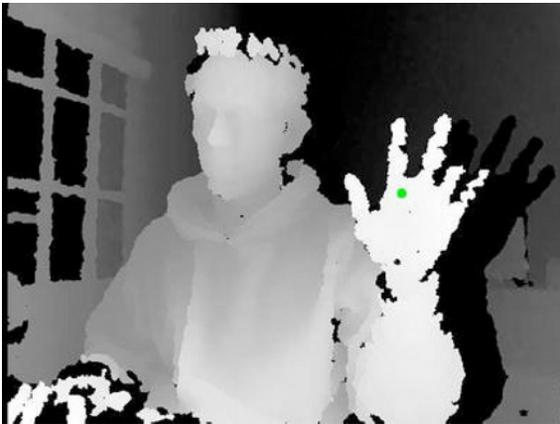
*Figure 4-7. Processing screen with hand tracking*
