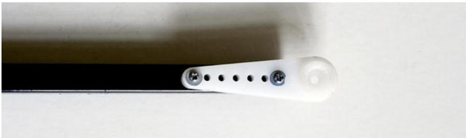
*Figure 13-2. Thigh connected to the servo horn*
