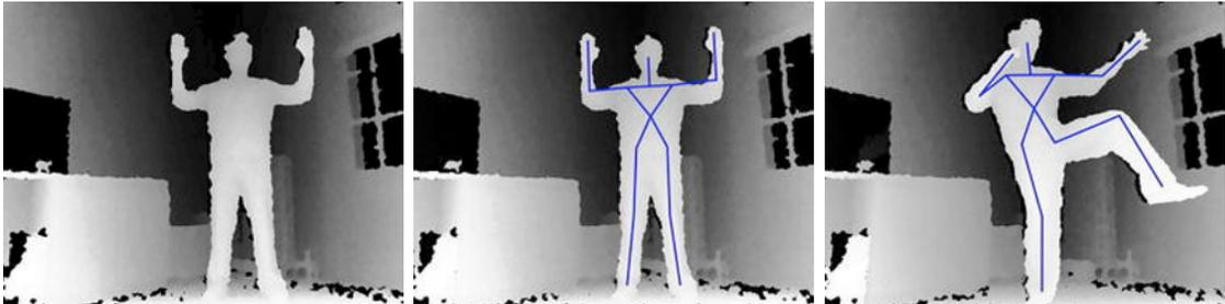
*Figure 3-13. User in start pose, calibrated, and tracked*
