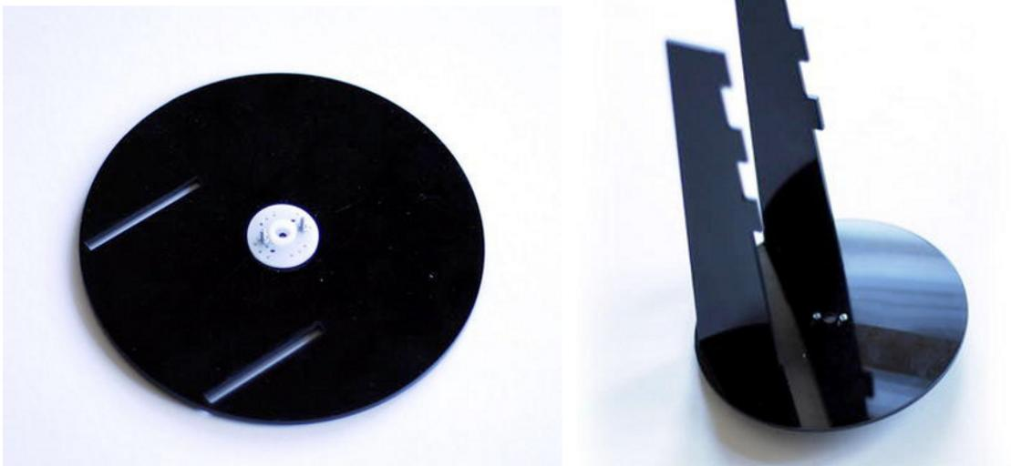
*Figure 6-6. Servo arm fixed to disc (left), and robot supports (right)*
