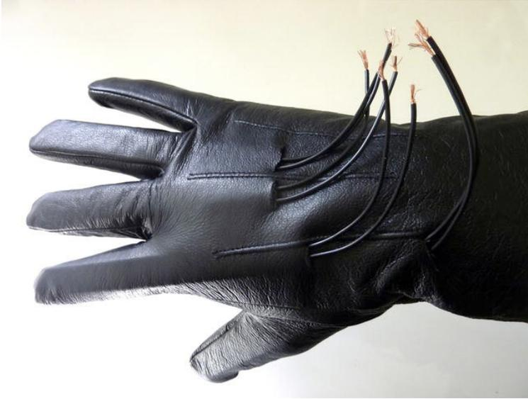
*Figure 11-7. Flex sensors installed in the glove*
