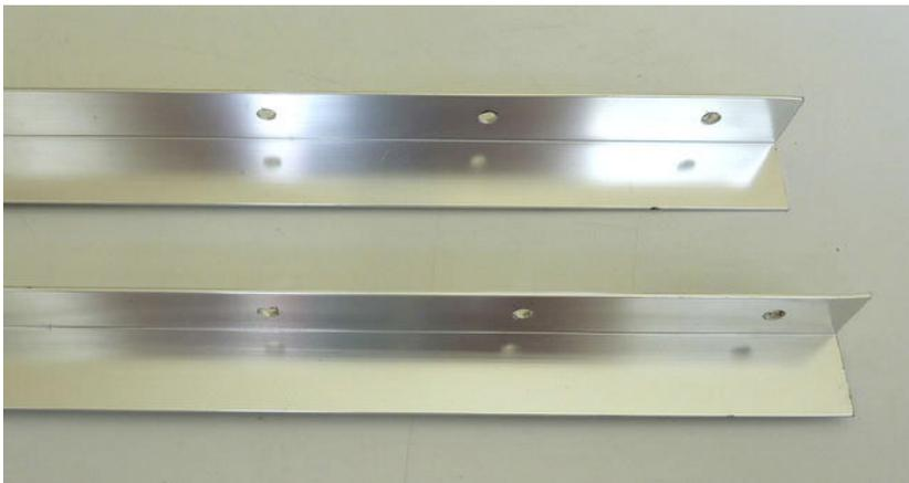
*Figure 12-13. Bracing aluminum angles after drilling the holes*
