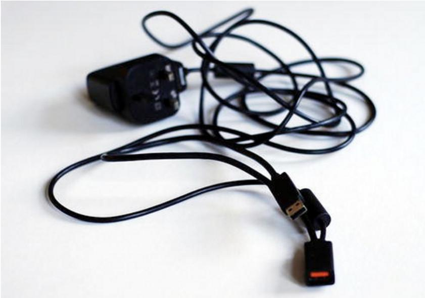
**Figure 2-2.** Kinect AC adapter with standard USB connection
