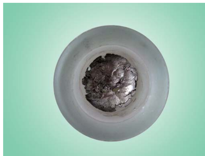
Fig. 9.10: Overtrituated mix sticks to be capsule which is difficult to remove
