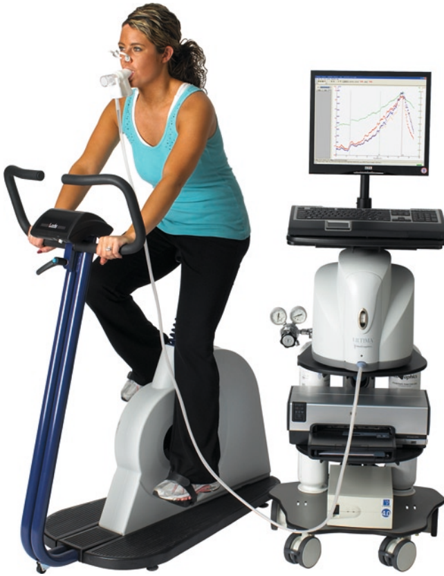
Fig. 4.1 Example of equipment needed to conduct a cardiopulmonary exercise test to measure peak oxygen uptake and other gas exchange parameters
