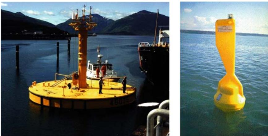
**Fig. 2** Examples of a moored (left) and drifting buoy (right) (images courtesy of NOAA National Data Buoy Center and the Data Buoy Cooperation Panel).
