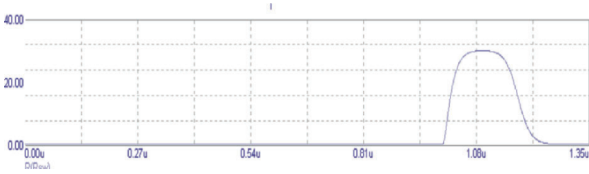
Fig. 12.21. Resistance of a plasma breaker versus time.
