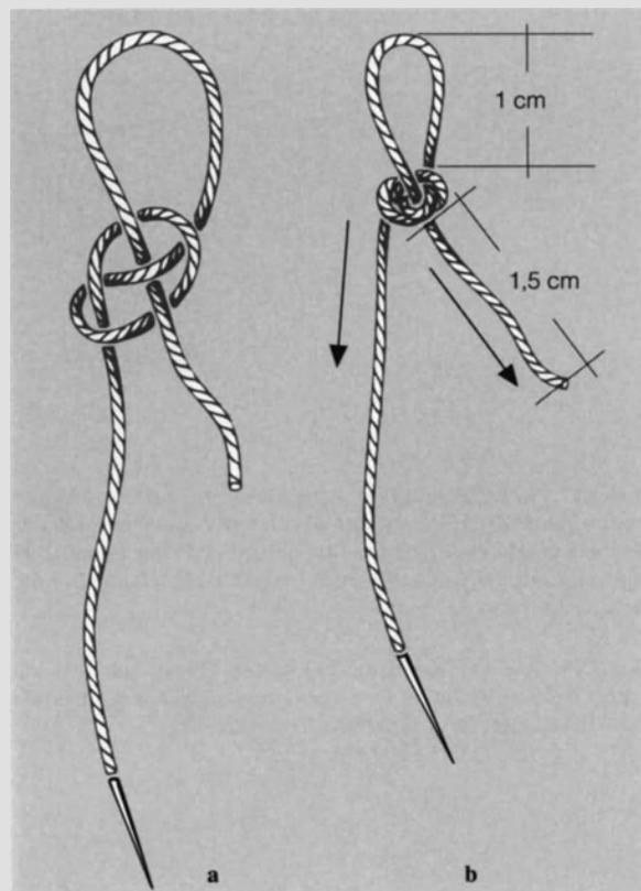
**Fig. 7.20 a, b.** When fashioned (a), the JSLK should be slipped from the tail to form a 1.0-cm bind or loop after which the tail is cut short (1.5 cm) (b)
