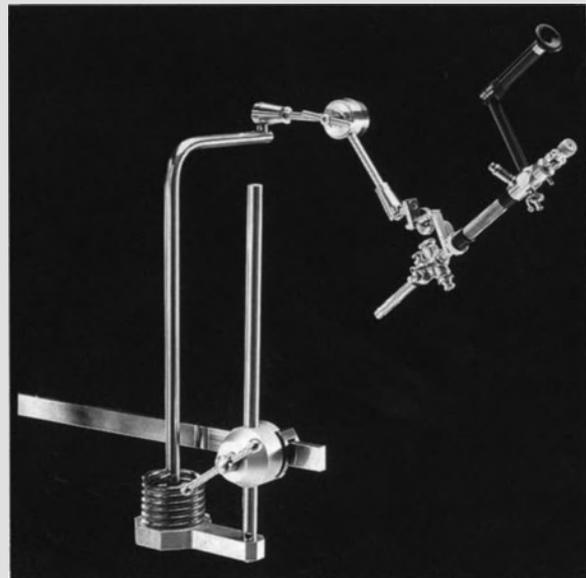
**Fig. 2.15.** Martin arm holding an endoscope
