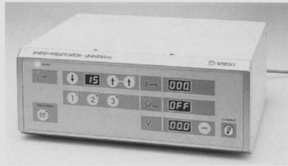
**Fig. 9.20.** A CO<sub>2</sub> insufflation unit with preset, electronically controlled insufflation pressure and dual electronic pressure limiter. Digital display of intracavitary pressure and flow (and of total filling volume). Touch switches are used to preset and adjust the parameters
