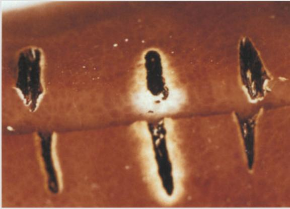
**Fig. 4.15.** Typical laser cuts in liver tissue achieved by 1, CO<sub>2</sub>; 2, Nd: YAG; 3, argon-ion laser radiation (from left to right)
