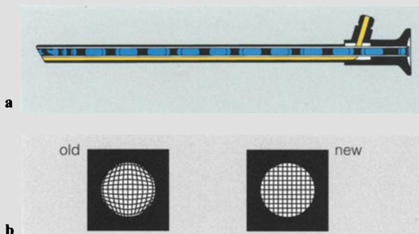
**Fig. 2.2.** a Longitudinal section of modern rigid endoscope (Panaview, Wolf). Light is reflected at the surfaces of air lenses and transmitted in glass rods. b Distortion of the borders of the image through the endoscope; *old*, conventional lens system; *new*, new lens system using image correction lenses (Olympus, Winter&Ibe)
