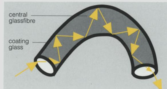
**Fig. 2.7.** Light passing through a glass fibre. On account of the lower diffraction index of the coating glass, the light is totally reflected
