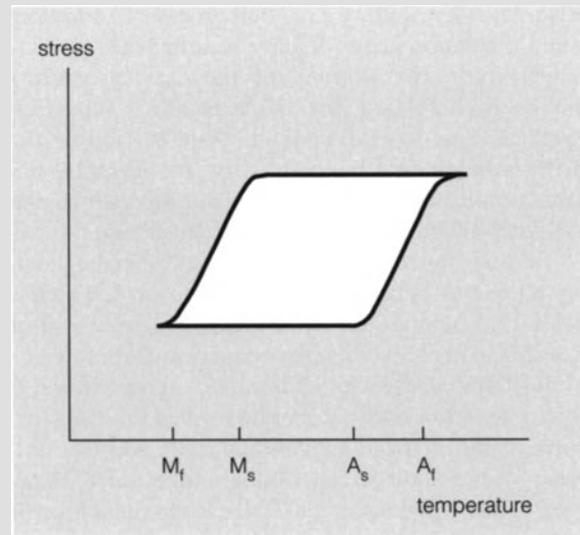
**Fig. 27.4.** The temperatures  $M_s$ ,  $M_f$ ,  $A_s$  and  $A_f$  define the thermal transformation hysteresis loop of the shape memory alloy
