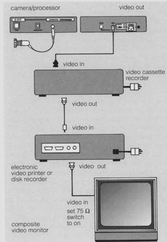
Fig. 3.5. Schematic diagram showing connections in video system
