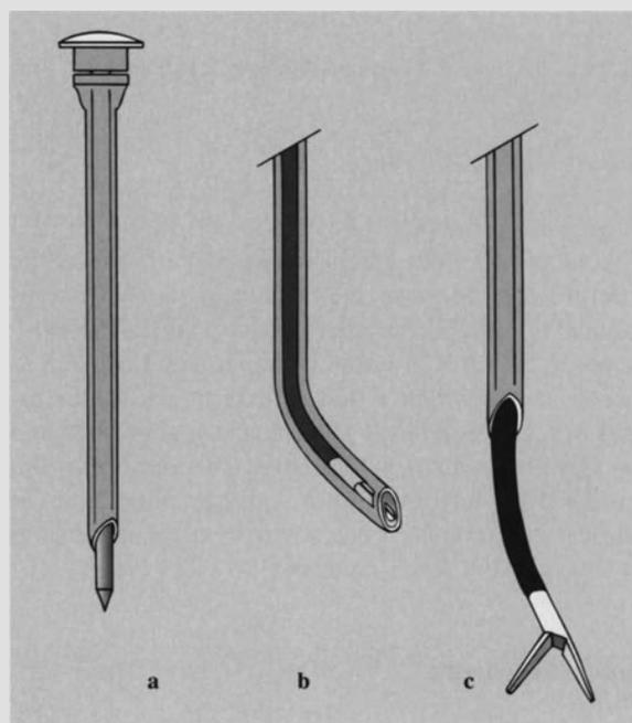
**Fig. 23.3.** **a** Flexible 5.5-mm trocar and cannula. **b** Cannula without metal trocar (Storz) with curved instrument being introduced. **c** Curved instrument after passage through flexible cannula
