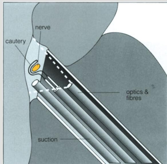
**Fig. 9.12.** Principle of tube dissection. With the telescope retracted, the end of the sheath provides a circumferentially shielded space for tissue dissection
