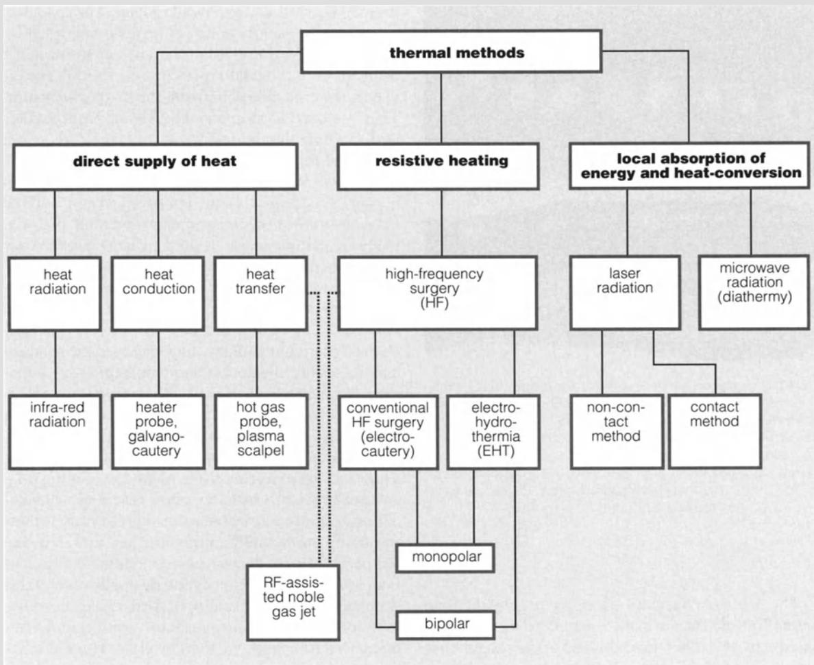
**Fig. 4.1.** Methods for the production of operative-therapeutic heat
