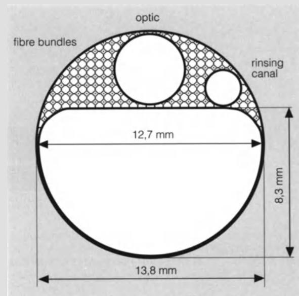
**Fig. 12.5.** A cross-section of the operating mediastinoscope. The working channel is an incomplete circle
