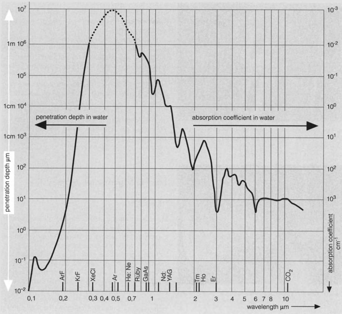
**Fig. 4.14.** Wavelength-dependent absorption and penetration depth of water and haemoglobin
