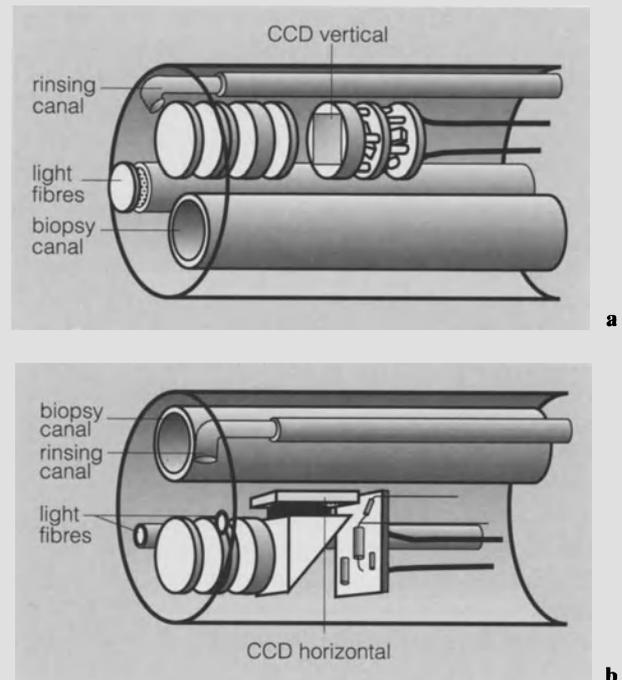
**Fig. 2.6 a, b.** The integration of the CCD chip into the tip of the endoscope. **a** Olympus, CCD vertical; **b** Fujinon, CCD horizontal
