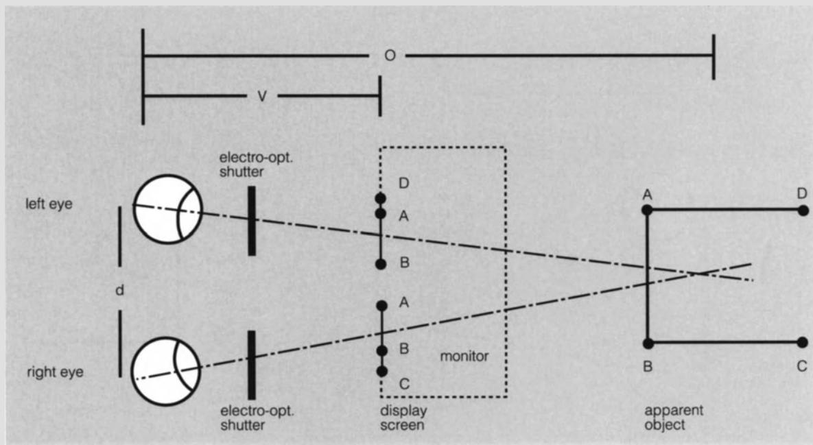
**Fig. 27.3.** Sequential display: in this instance, the TV monitor serves as the medium for the projection of the virtual images being recorded by the two cameras with sequential display of left- and right-eye information (100 or 120 Hz)
