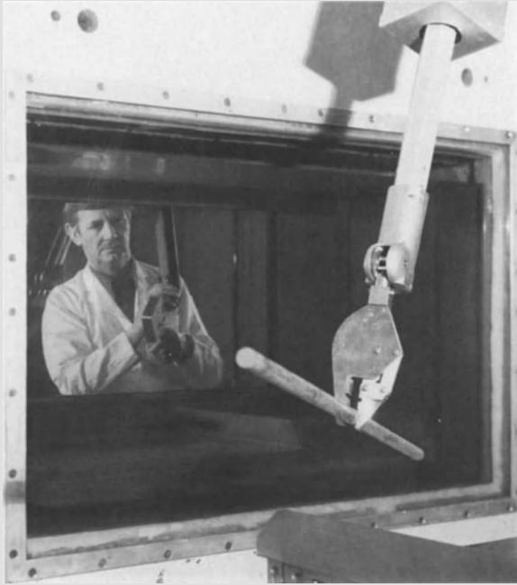
**Fig. 27.11.** Master-slave manipulator in a hot cell
