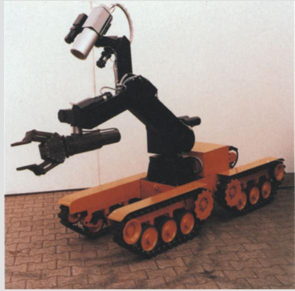
**Fig. 27.12.** Vehicle with power manipulator
