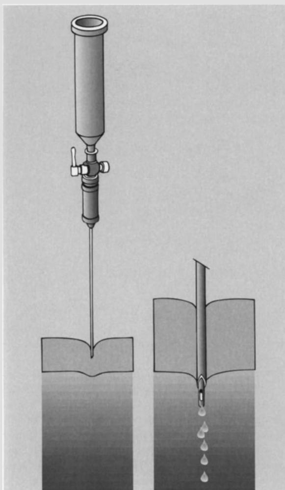
**Fig. 16.4.** The syringe safety test with saline
