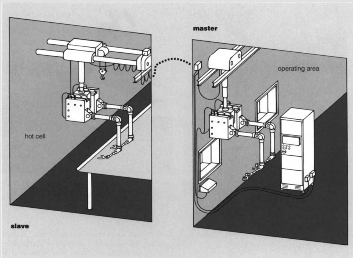
**Fig. 27.10.** Master-slave manipulator in a hot cell with shielding windows
