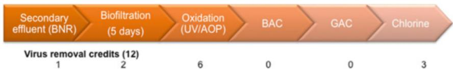
**Fig. 4** Virus log removal efficiency by a potable water reuse treatment train consisting of biofiltration via subsurface treatment, advanced oxidation, and activated carbon treatment followed by final disinfection prior to blending with conventional supply
