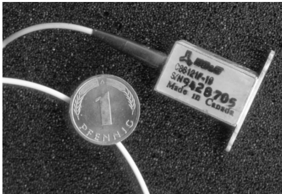
Figure 8.28: A laser diode made for communication purposes. This device is enclosed in a housing which must be bolted to a heat sink with the flange visible on the right, in order to remove heat. The electrical connections are by pins on the bottom and are not visible in this picture. The optical output goes into a piece of fiber attached to the laser (the pigtail). The pigtail is protected with a plastic coating and a rubber bend relief where it leaves the case.
