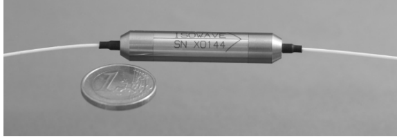
Figure 8.11: An optical isolator. It comes with two fibers attached, known as “pigtails”. The engraved arrow indicates the forward direction. A 1 Euro coin is shown for size comparison.
