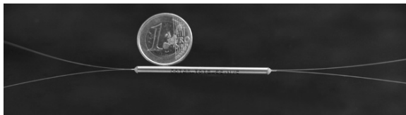
Figure 8.15: A typical fused fiber coupler. It comes with four pigtails.
