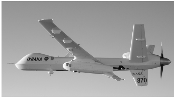
Figure 12.9: NASA's Ikhana, a modified Predator B unmanned aircraft adapted for civilian research, is being used to test advanced, fiber optic-based sensing technology to monitor structural integrity. Six fibers on the wing's top surface provide more than 2,000 strain measurements, thus providing full information of the wing shape in real time. They add merely 1 kg of weight and do not appreciably affect aerodynamics. The data gathered improve safety, but the ultimate goal is to develop active control of wing shape so that the aerodynamics can be adapted to take-off, cruising, and landing. Such capability could dramatically improve efficiency and performance. From [5].
