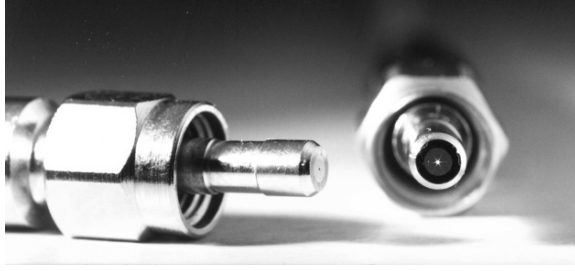
Figure 8.3: A typical fiber connector. At the center of the ferrule, one can see the fiber either as a dark or a bright spot, depending on lighting conditions.
