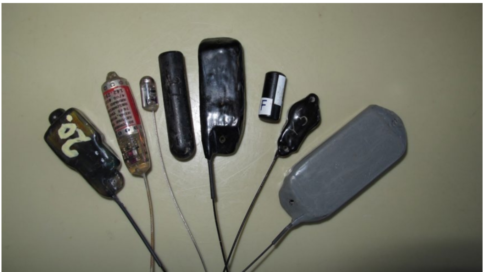
Figure 17.4 A collection of different radio and acoustic transmitters used to tag fish. The radio transmitters are those having an antenna, whereas the two cylindrical transmitters without antennas are acoustic transmitters. Acoustic transmitters usually have a cylindrical shape, whereas radio transmitters are produced in both cylindrical and flat shapes. A cylindrical shape is optimal for surgical implantation of transmitters, whereas a flat shape is optimal for external attachment to the fish. Photo: Eva B. Thorstad.
