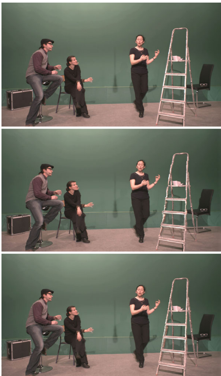
Fig. 4.17 Visual comparison of reconstructed view 3 with disparity map encoded at 450 kbps, sequence “Actors” ( top : original frame, middle : two disparity maps per view, bottom : enhanced disparity map per view)
