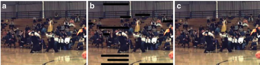
Fig. 12.11 Frame 0 of the Ballroom sequence [14] transmitted using a 150 byte slice size. (a) Original frame, (b) received frame assuming a packet error rate of 5 %, and (c) the displayed frame after applying spatial concealment
