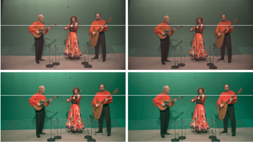
Fig. 4.7 Visual effect of the color and geometrical correction on cameras C_1 and C_2 ( top : before rectification, bottom : after rectification)
