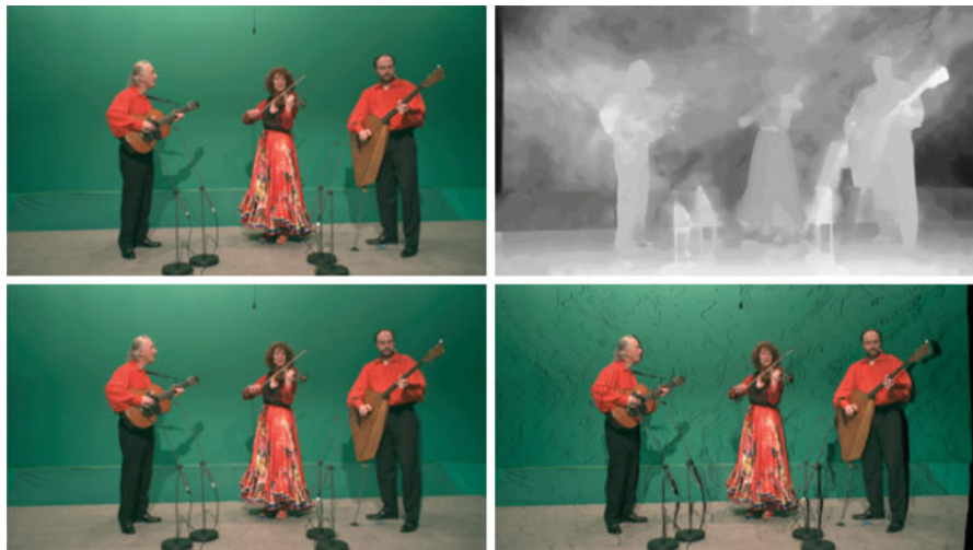
Fig. 4.12 Disparity map and view synthesis with accurate local block matching ( top left : original view 3, top right : disparity map, bottom left : synthetised view 3 with inpainting (32.81 dB), bottom right : synthetised view 3 with 5 % of occluded pixels)
