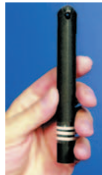
Mini-Armour Ophthalmoscope—a simple pen torch with attached basic optical system. (Courtesy of Roger Armour)
