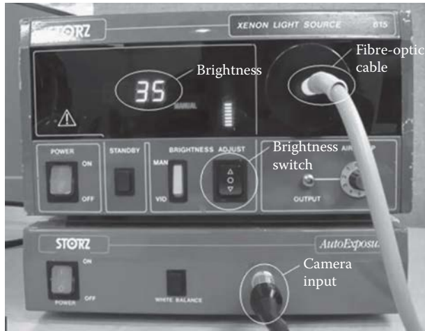
FIGURE 2.1 A typical source of light for endoscopic viewing. The light source is transmitted through a fiber-optic bundle mounted around the endoscope to the surgical site. The light source also allows adjustment of the illumination conditions to be set.
