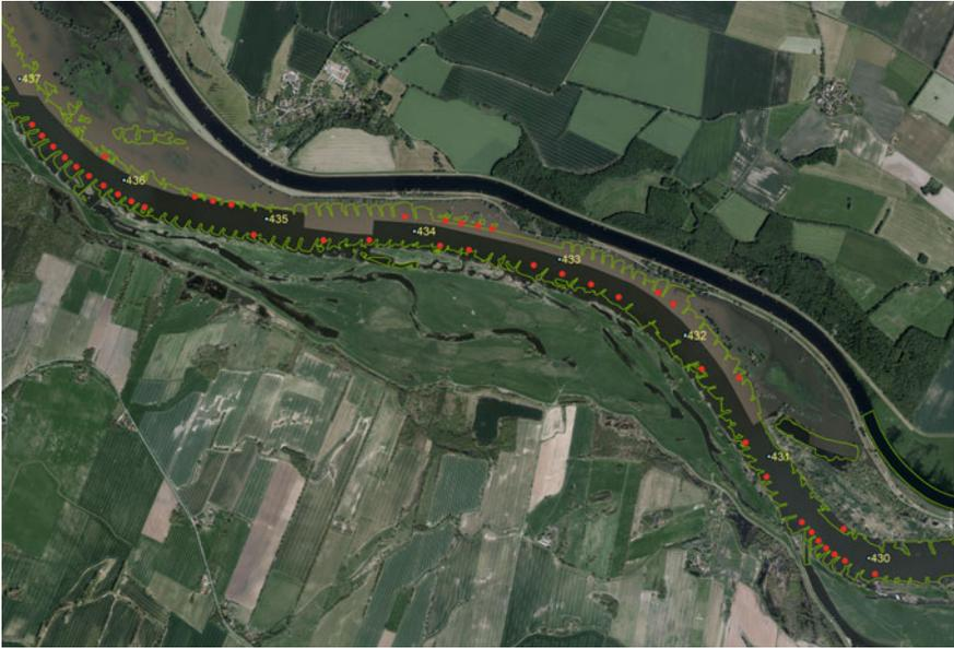
**Fig. 3** Aerial survey of the Elbe (DE-km 430–437). *Source* Federal Agency for Cartography and Geodesy (BKG) and Federal Institute of Hydrology (BfG). *Red spots* groyne fields with contaminated fine sediments
