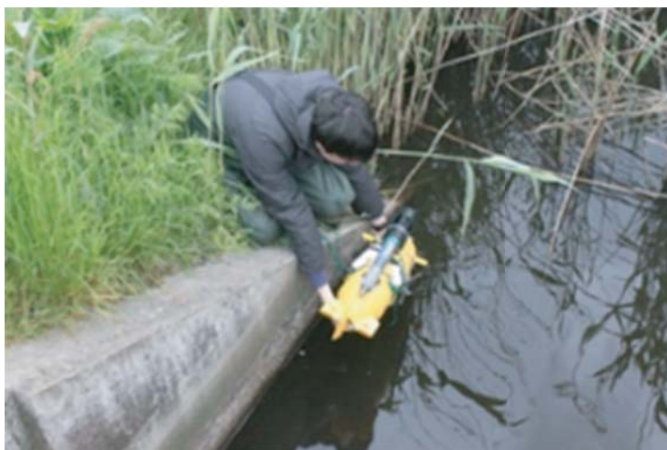
Figure 23.14 Aqua drones used for water quality and ecoscans as applied in Hoogeveen wetland [16]. Reproduced with permission.
