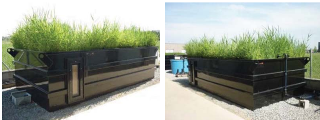
Figure 21.8 Phragmites in the pilot VFCW.
