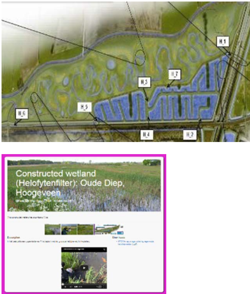
Figure 23.9 Example of one of the largest horizontal flow wetlands in Hoogeveen; top view of the wetland (left), information of this wetland (right) ( http://www.climatescan.nl/page?details=91 ).
