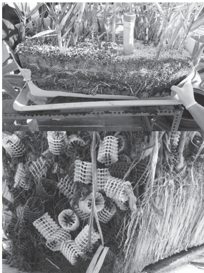
Figure 9.4 Photo of the HDPE substrate material in the pilot wetland units.
