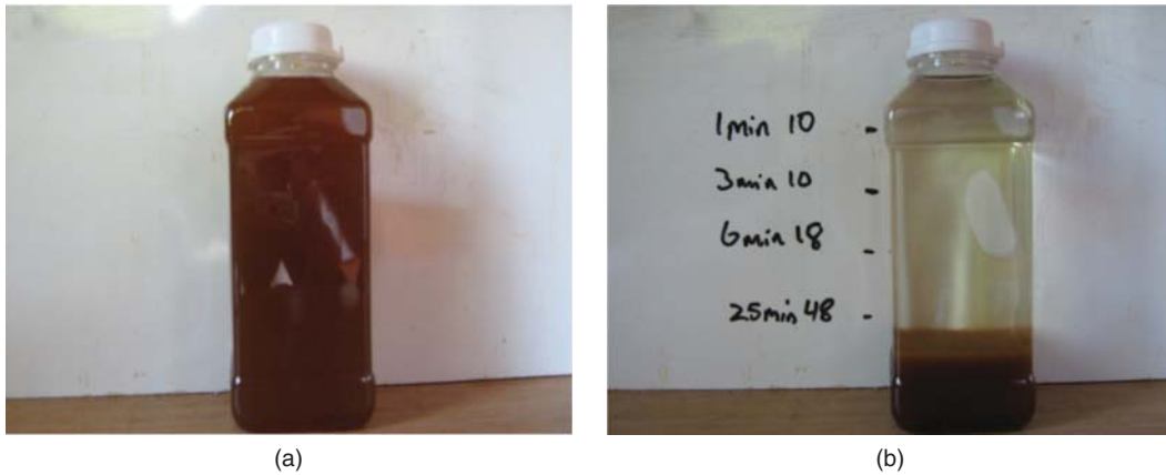
Figure 19.10 Sedimentation of Hanningfield WW sludge performed on sludge sampled 28.07.2009 (Photo: Orbicon).
