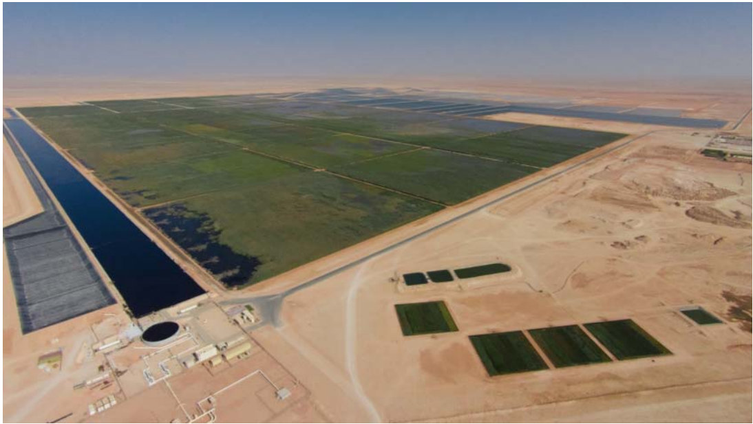
Figure 1.4 Aerial view of the inlet buffer pond and the SFCW cells. [4]
