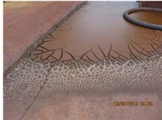
Figure 19.13 Examples of the sludge surface in Whitacre Test system. Pictures are taken 21 days after the last load (left) and 1 day after the load (right). Note the evident cracks in the sludge after only 1 days' rest (Photo: Orbicon, reproduced with permission).
