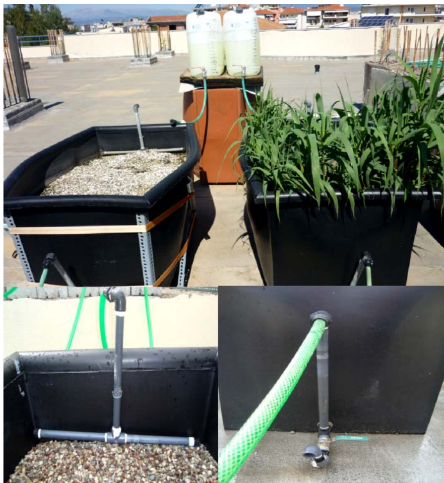
Figure 9.3 Pilot-scale HSF CWs for the treatment of Cr(VI) and SCW (upper two photos); perforated inflow pipes (diffuser) (bottom left photo); outlet tube of the CWs (bottom right photo).
