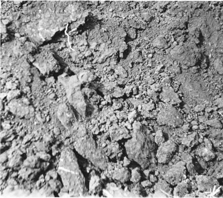
FIGURE 30. Gypsum and lime veinings cement soil particles together. (From Fuller, W. H., Management of Southwestern Desert Soils , The University of Arizona Press, Tucson, 1975.)
