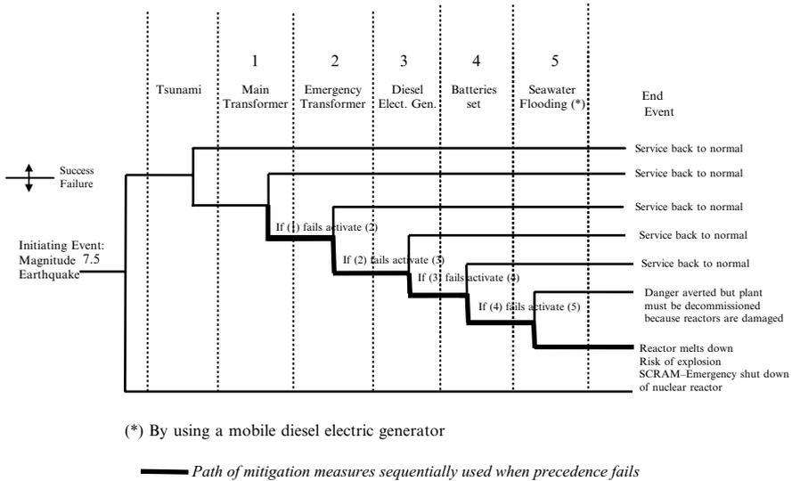
**Fig. 5.16** Events tree for water pumps in a nuclear power plant
