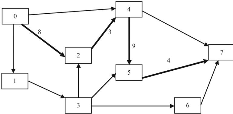
Fig. 3.1 CPM network using deterministic values for durations
