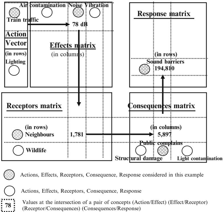
Fig. 4.3 The Z-Matrix for an urban rail system
