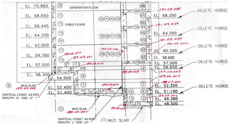
Fig. 8.1 Actual concrete work done for hydroelectric turbine installation
