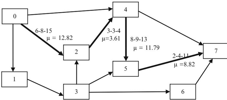
**Fig. 3.3** Network with mean values from Monte Carlo for durations
