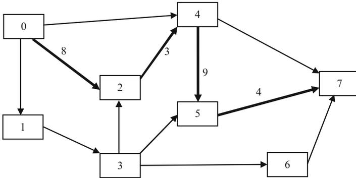
**Fig. 2.1** CPM network using deterministic values for durations
