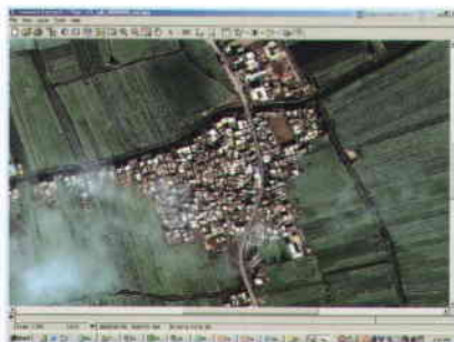
IKONOS satellite image, multi-spectral, 1 m resolution, 1:5000 scale, Aba-Masoud, Egypt
