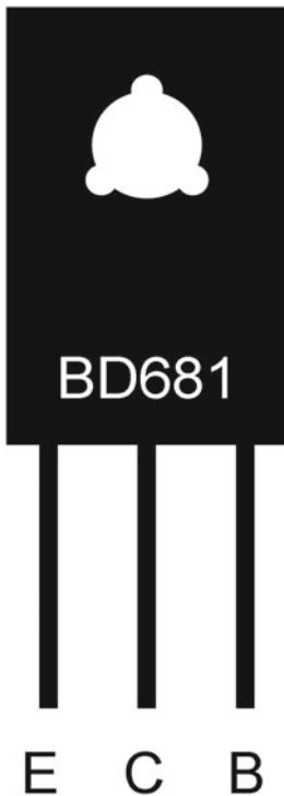
**Figure 4-20.** *BD681 Darlington Transistor pinout*
