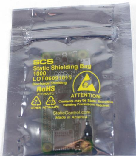
**Figure 1-10.** Warning symbol for a static-sensitive component
