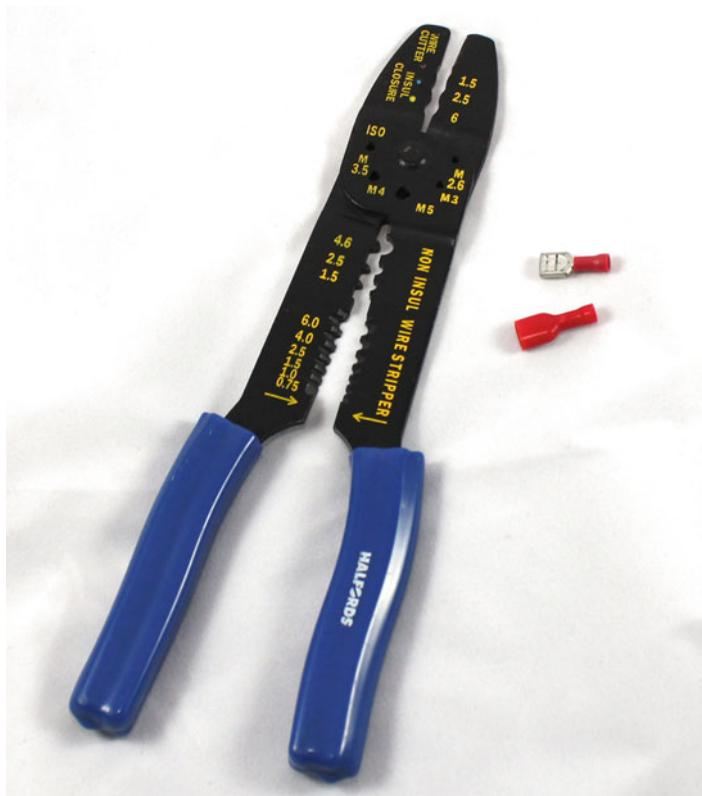
**Figure 3-23.** Crimp tool with female blade connectors
