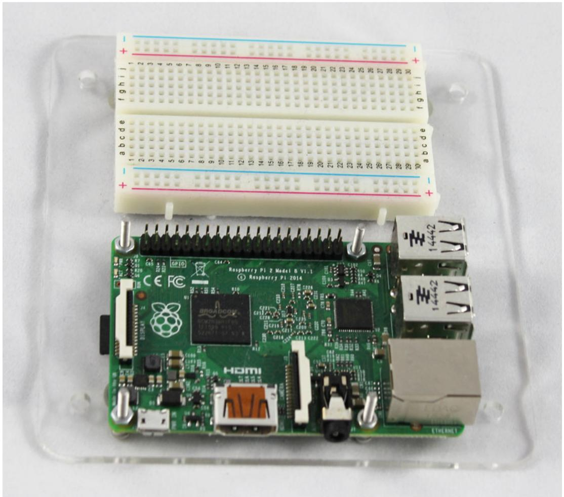
**Figure 1-5.** *Raspberry Pi and a breadboard mounted together*
