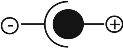
**Figure 4-4.** DC power adapter center positive indicator
