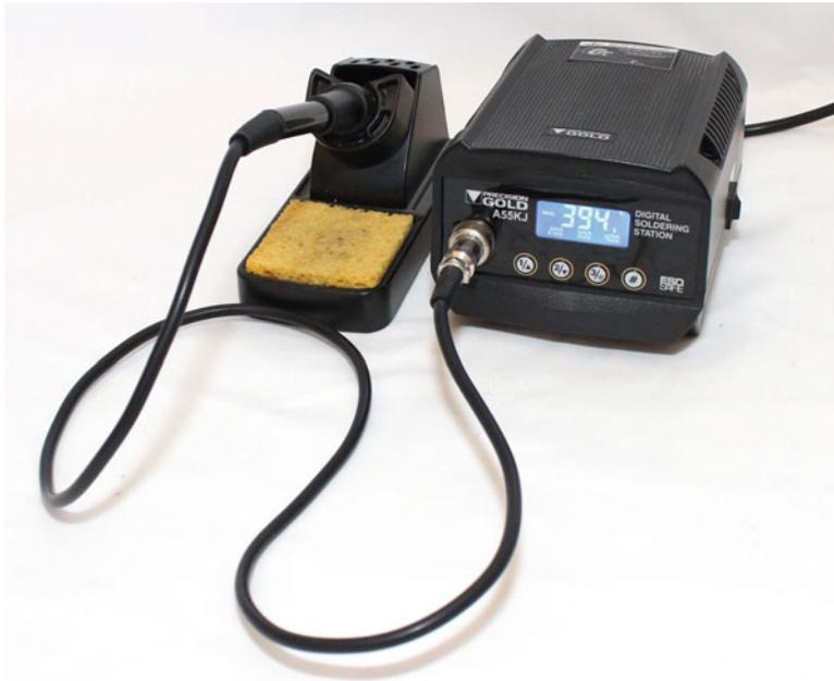
**Figure 10-1.** Temperature controlled soldering iron
