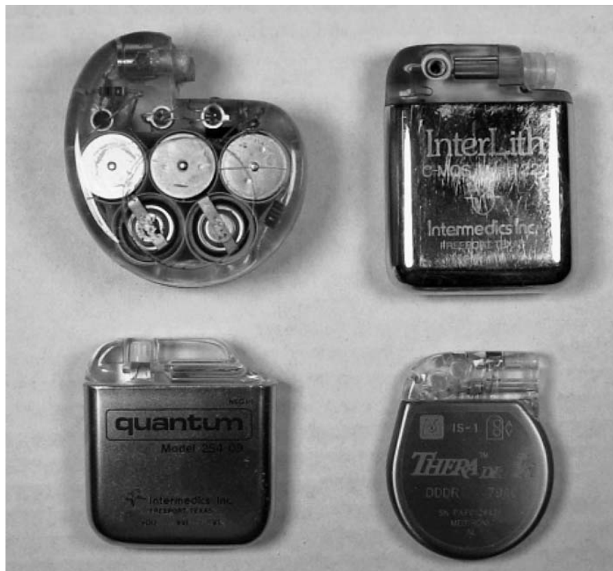
Figure 8.8 Evolution of implantable pacemakers. Top, left to right: Very early CCC VOO pacemaker powered by six mercury cells, Intermedics InterLith VVI with CMOS circuitry and powered by a lithium cell. Bottom: Intermedics “Quantum” programmable VVI/VVT pacemaker, a modern Medtronic Thera DDDR pacemaker.
