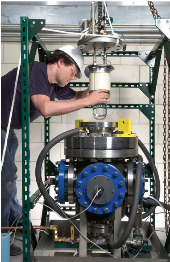
Fig. 5.25 At the heart of the COUPP detector is a small bubble chamber, shown here removed from and situated above its outer casing. (Image courtesy of Fermi Lab)
