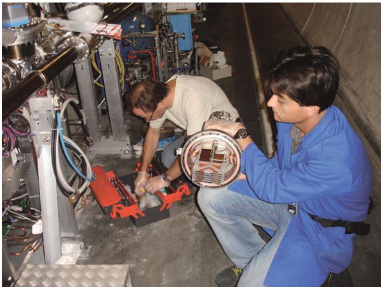
Fig. 2.26 Technicians work to install one of the “Roman pots” that will be used in the TOTEM experiment. (Image courtesy of CERN)
