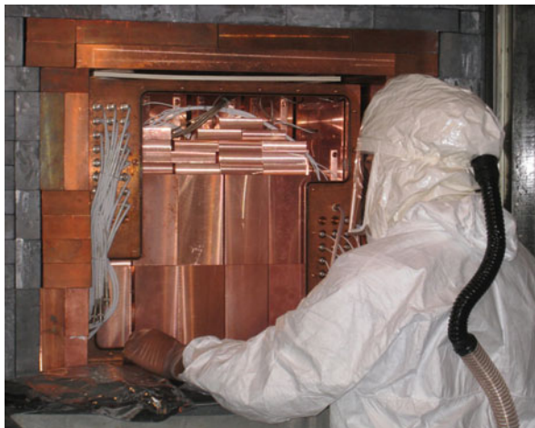
Fig. 5.23 A technician inspects the copper and lead shielding that surrounds the sodium iodide detectors at the heart of the DAMA/LIBRA experiment. (Image courtesy of the LNGS)
