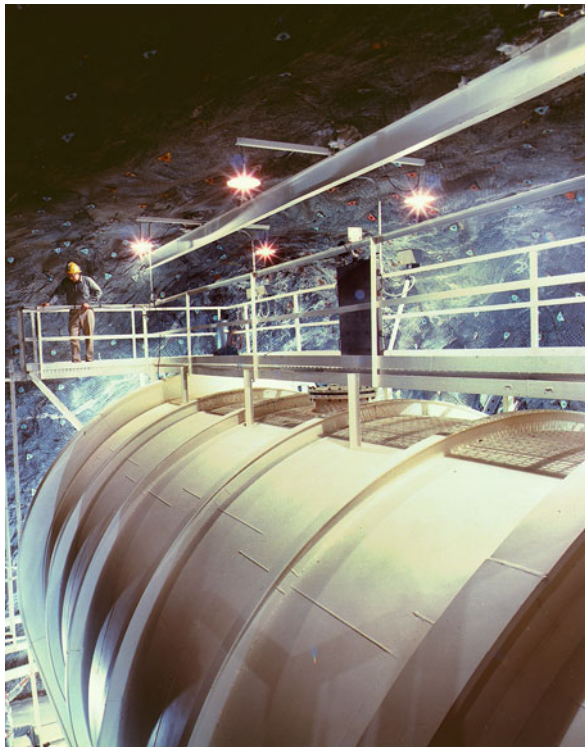
Fig. 1.17 The large tank containing 455,000 liters of dry cleaning fluid – the liquid heart of the Homestake Mine solar neutrino experiment. (Image courtesy of the Brookhaven National Laboratory)
