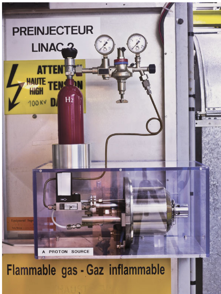
Fig. 2.7 The hydrogen supply cylinder – the starting point of the LHC experiment. At full beam loading about 2 ng ( 2 \times 10^{-12} kg) of hydrogen will be consumed by the LHC per day. (Image courtesy of CERN)
