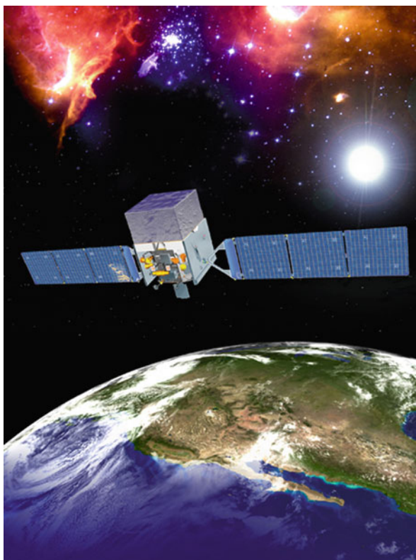
Fig. 5.28 An artist’s impression of the Fermi Gamma-Ray Space Telescope. In addition to surveying the sky at gamma-ray wavelengths, the detector aboard the spacecraft will look for signals relating to dark matter annihilation events. (Image courtesy of NASA)
